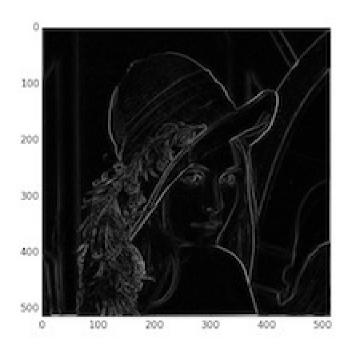
You can think of Gx and Gy as sort of like vectors, so we can calculate the magnitude and direction. So  $G = \operatorname{sqrt}(Gx^2 + Gy^2)$ . We can see that after applying both operators what we get out is all the edges detected.
