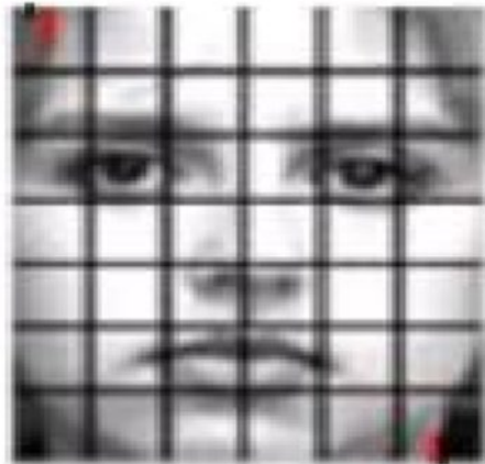
Figure 12-3. Applying LBPH for face recognition starts by dividing the face image into a 7x7 grid of equally sized cells
