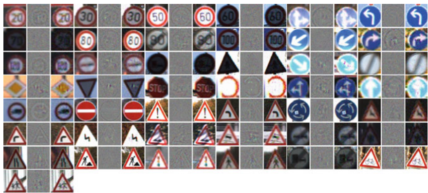
Fig. 5.18 Minimum additive noise which causes the traffic sign to be misclassified by the minimum different compared with the highest score
