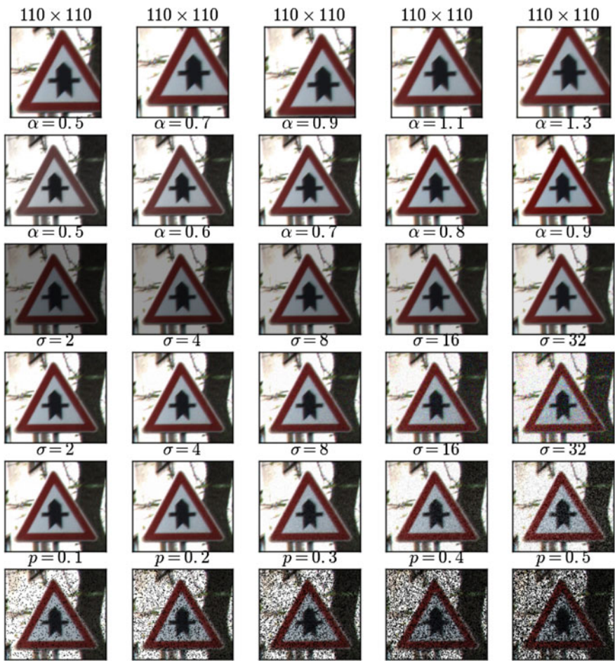
Fig. 5.5 Augmenting the sample in Fig. 5.4 using random cropping ( first row ), hue scaling ( second row ), value scaling ( third row ), Gaussian noise ( fourth row ), Gaussian noise shared between channels ( fifth row ), and dropout ( sixth row ) methods with different configuration of parameters
