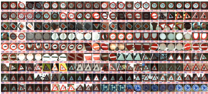
Fig. 5.16 Incorrectly classified images from the BTSC dataset. The blue and red numbers below each image show the actual and predicted class labels, respectively. The traffic sign corresponding to each class label is illustrated in Table 5.5
