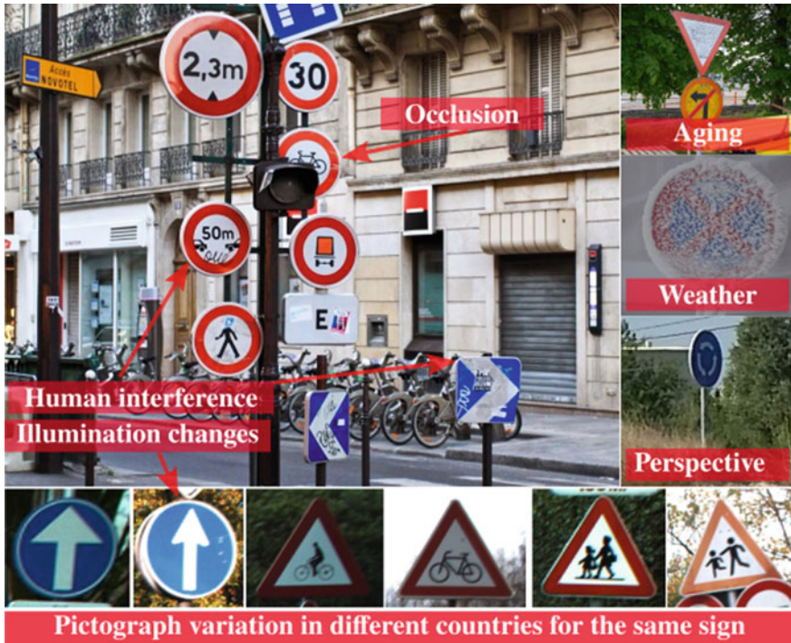
Fig. 1.2 Some of the challenges in classification of traffic signs. The signs have been collected in Germany and Belgium
