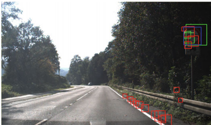
Fig. 6.3 Applying the trained ConvNet for hard-negative mining
