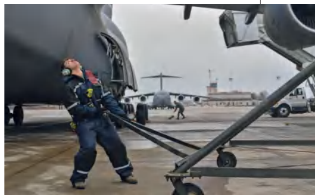
A crew chief, pulls a maintenance platform up to a C-5 Galaxy at Ramstein Air Base, Germany. Airmen assigned to the 721st Aircraft Maintenance Squadron marshal aircraft to parking, chock the wheels, hook-up generators, check tyre pressures, refill oil, and refuel the aircraft. Senior Airman Tryphena Mayhugh/US Air Force
