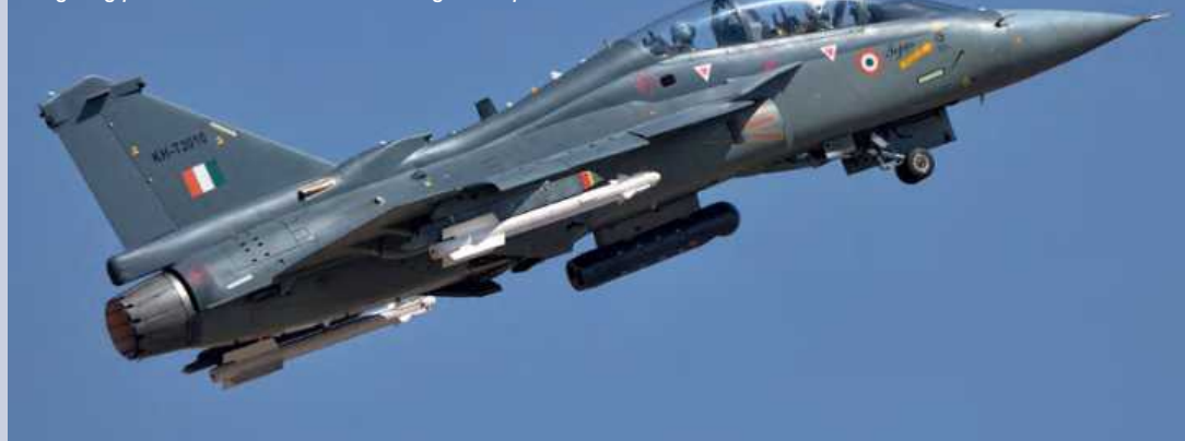
Two, two-seat Tejas fighters flew customer orientation and familiarisation flights during the show. Note the Israeli Litening targeting pod carried on the under-fuselage hard point.
