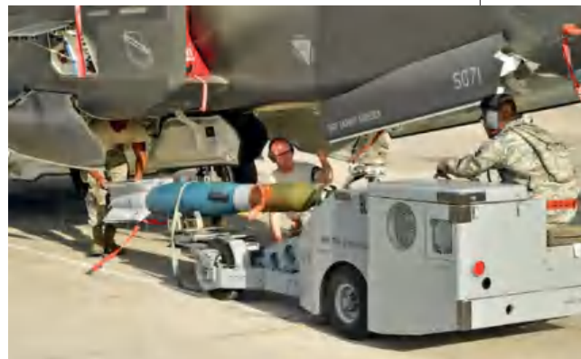
A weapons load crew assigned to the 34th Aircraft Maintenance Unit based at Hill Air Force Base, Utah, loads a GBU-12 into an F-35A Lightning II.
