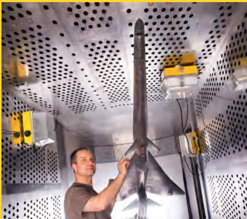
Mechanical technician Dan Pitts prepares the 9% scale model of Lockheed Martin's Quiet Supersonic Technology X-plane preliminary design for its first high-speed wind tunnel tests at NASA's Glenn Research Center. NASA
