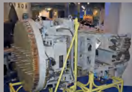
The NIIP N011M Bars electronically scanned array radar features three rows of small T-shaped antennas in the centre for the IFF. Piotr Butowski
