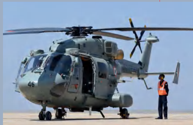
Top Left: HAL's Weapon System Integrated Advanced Light Helicopter (WSI ALH) MkIV Rudra, the combat version of the Dhruv, received its initial operational clearance in February 2013 and is now in production. Top Right: Dhruv ZD-4146, is a rare example of an Indian Air Force Dhruv configured with a wheeled retractable tricycle landing gear. Most are equipped with skids; wheels are typical for the Navy's variant. This variant is equipped with a self-protection suite similar to the system fitted to the Rudra.
