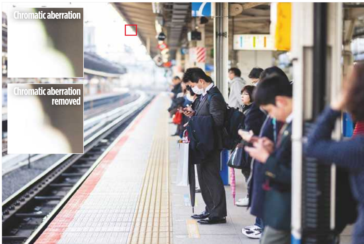
Evidence of minor fringing can be seen above. Canon EOS 5DS R, Sigma 85mm f/1.4 DG HSM Art, 1/640sec at f/1.8, ISO 200
