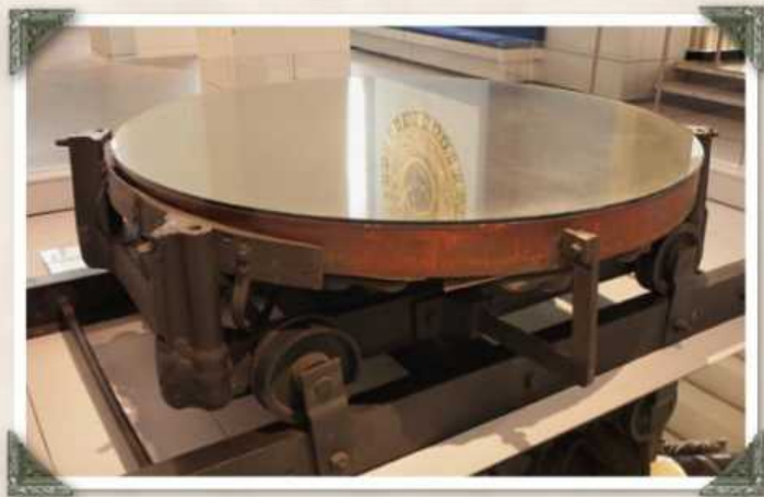
Left: The “Leviathan of Parsonstown,” a 72-inch reflector, was constructed in 1845 by William Parsons, third Earl of Rosse. Right: One of the original speculum (copper and tin) mirrors is on display in the Science Museum in London. WIKIMEDIA COMMONS
