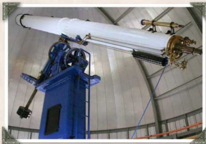
Above: "Rachel" is a 20-inch refractor created by Warner & Swasey with optics by noted lens-maker John Brashear. This telescope, located at the Chabot Space & Science Center in Oakland, California, is the largest refractor in the western U.S. regularly open to the public. MIKE REYNOLDS
