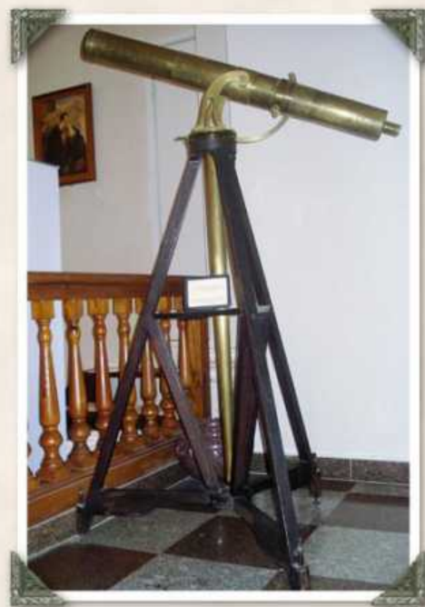
This 4-inch refracting telescope by John Dollond resides in the White Hall of the Vilnius University Library in Lithuania. Dollond made only the scope; another craftsman made the tripod.
