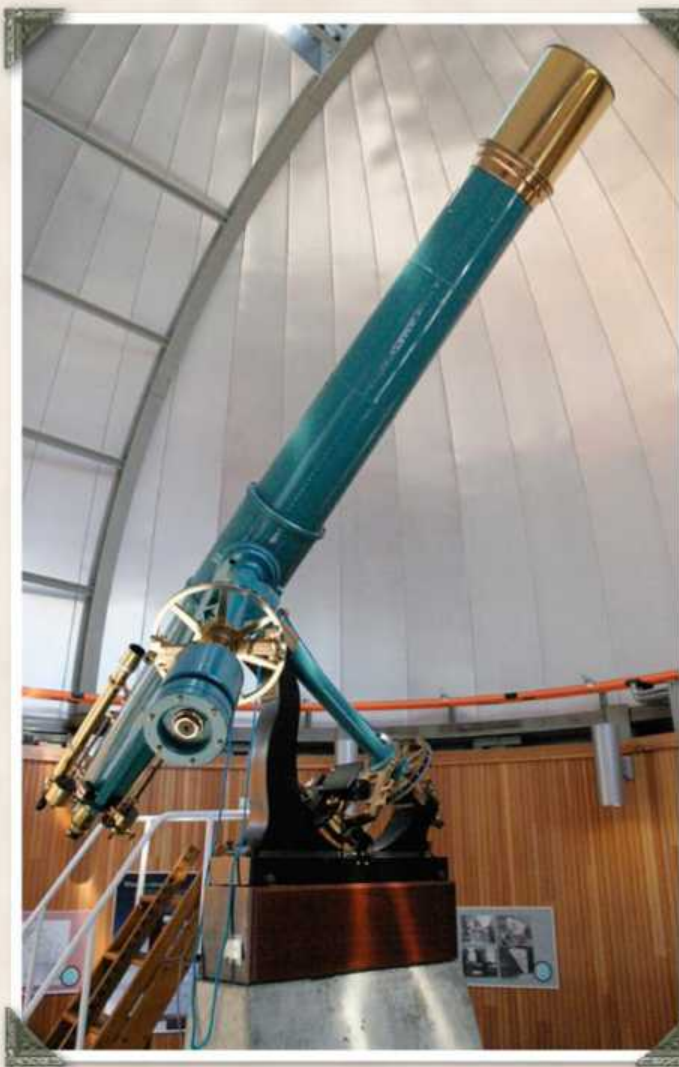
Above: "Rachel" is a 20-inch refractor created by Warner & Swasey with optics by noted lens-maker John Brashear. This telescope, located at the Chabot Space & Science Center in Oakland, California, is the largest refractor in the western U.S. regularly open to the public. MIKE REYNOLDS
