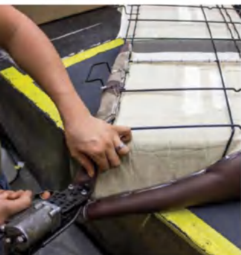
16 | The covers are pulled over the foam and attached to the seat frame with an upholstery-specific staple gun.
