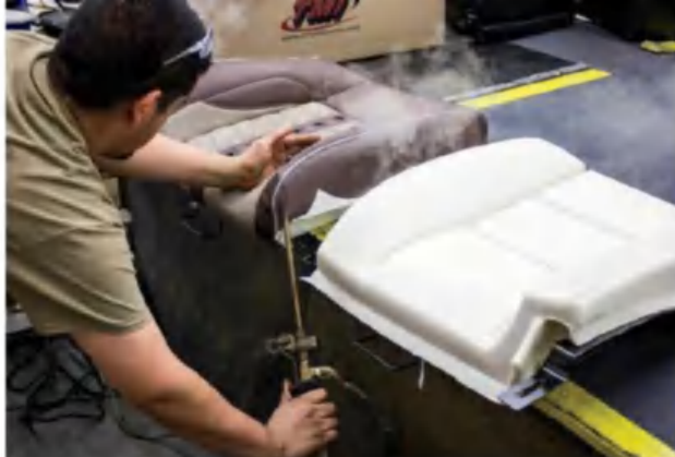
15 | A steamer is used to soften the leather, making it easier to stretch over the foam and get rid of unwanted creases.
