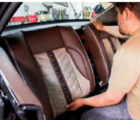
17 | With the seat frame notched to clear the wheelwells, each seat assembly slides into place.
