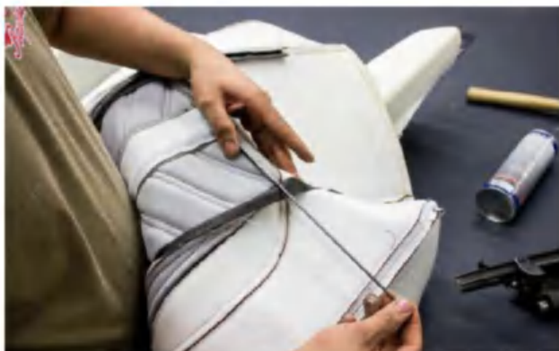
14 | Thin steel rods are cut and inserted into slots in the underside of the seat covers. These serve as mounting points to attach to the frame.
