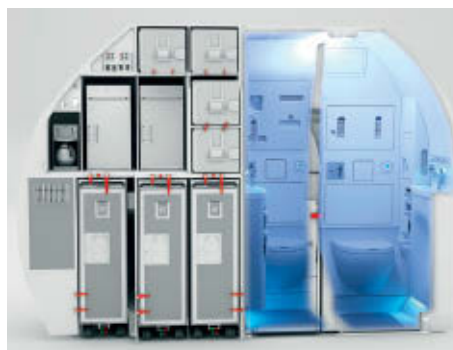
The Space-Flex v2 rear galley and lavatory module for A320s, produced by Zodiac
