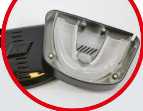
Devices like the FitGuard can track collisions and help to alert players to injuries instantly
