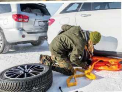
BLOWING HOT AIR The Bushranger X-Jack is supposed to use a vehicle's exhaust to inflate a heavy-duty rubber jack. After inhaling too much exhaust, we opted for a standard jack.
