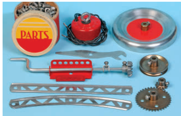
FIGURE 4. Here are several typical parts including a 5" girder, 5" curved girder, 3" disc wheel, and a cool electromagnet.
