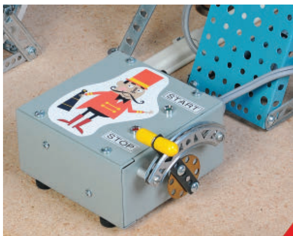
FIGURE 8. My start/stop lever switch emulates the manual clutch lever used on old-fashioned carnival rides.
