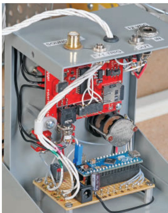
FIGURE 10. The red SparkFun triggerable MP3 board plays carnival music to give the project the feel of the midway.
