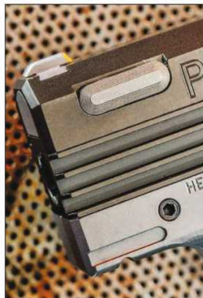
Turning the lever on the left side of the slide, near the muzzle, allows you to remove the recoil spring assembly during the takedown process.
