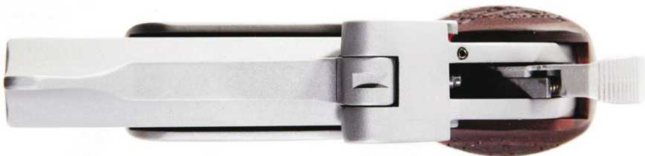
The front sight is a large ramp, and the rear sight is a square notch on top of the barrel hinge.
