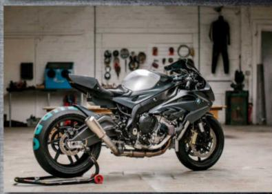
finishing touches include coating the Öhlins fork internals in black ceramic to match the bike's colour scheme, a carbon fibre swingarm wrap and wheels from a BMW's limited HP4, while the rearsets, clip-ons and braided lines were sourced from Bonnamici.
