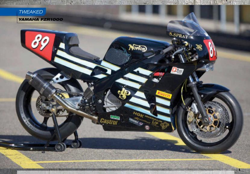
to ride. More than a few kilos were taken off the crank to lighten it, a 12:1 compression ratio Wiseco 1040cc big bore kit was fitted, and a YZF750 six-speed gearbox sourced to replace the standard five speed. For the top end goodness Shaun ported the head with his top-secret design, kept the standard camshafts for the moment and slipped on a set of Keihin 39mm flat slide carbs. The size of the carbs was a hotly debated subject but Shaun said he wanted 39s and not 41s so that's what he got.
