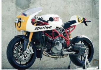
Rob North machines in the modern linkage rear shock. Rosell said he had to modify the swingarm so the 5.5-inch wide Daytona rear wheel would fit, while XTR Pepo parts have also been used or custom-fabricated for the adjustable levers, clip-ons, fairing, front bracket, screen, seat, rear guard and rearsets.
