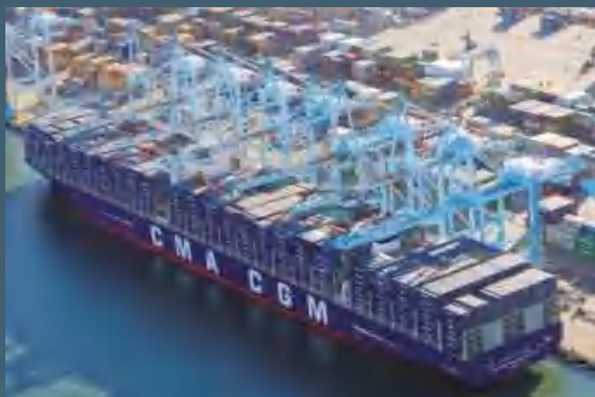
▲ The capacity of several new container ships has now gone over 20,000TEU, and ships of 26,000TEU are on the drawing board, but shoreside handling capacity and logistics may limit their future growth. CMA CGM
