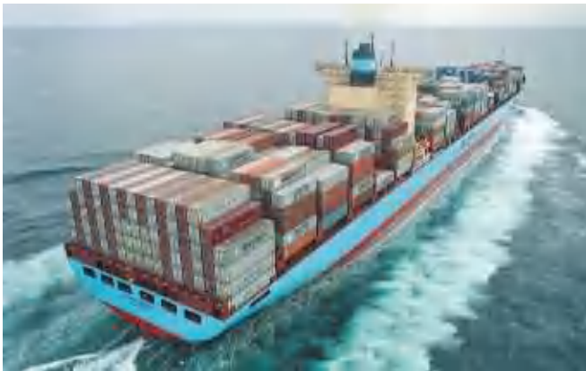
▲ One of the many container ships transiting the English Channel, the 98,648gt Gudrun Maersk was photographed in August 2005 when new. Constructed at the Odense Steel shipyard in Denmark, when launched in 2005 she was the world's largest container vessel, capable of carrying up to 8,500TEU, a title she lost in 2006 to Emma Maersk.
