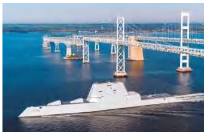
▲ Zumwalt passes under the Chesapeake Bay Bridge and heads seawards away from Baltimore on 17 October 2016. The two AGS Advanced Gun Systems can be seen forward of the bridge and a Fire Scout unmanned aerial vehicle is on the flight deck. ALL PHOTOS BY US NAVY
