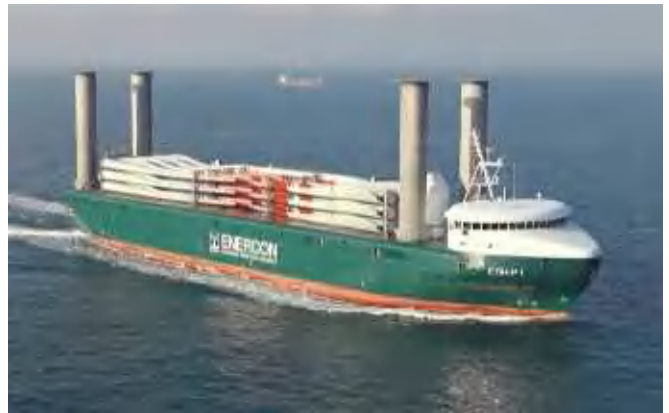
▲ Owned by the world's third largest wind turbine manufacturer, Germany's Enercon GmbH, the 10,500dwt ro-ro vessel E-Ship 1 makes use of four Flettner rotors, first developed in the early 1920s, along with two diesel engines of 7MW combined output. She is employed to deliver wind farm components worldwide, and has a service speed of 16.5 knots.
