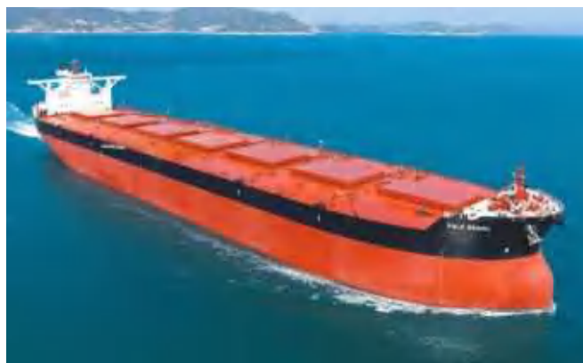
▲ Completed by South Korea's Daewoo Shipbuilding & Marine Engineering Co in 2011, the 402,347dwt Valemax ore carrier Vale Brazil measures 1,187.7ft (362m) by 213.3ft (65m) and is propelled by a single MAN B&W 7S80ME-C8 engine driving a fixed pitch propeller to give daily fuel consumption of 96.7 tons at 15.4 knots. DS&ME
