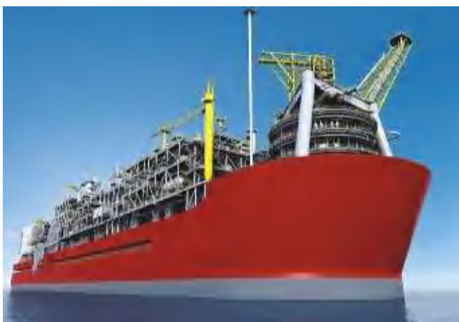
▲ The 300,000gt Prelude, the world's first floating liquefied natural gas (FLNG) platform, and the largest offshore facility ever built, measures 1,601ft (488m) by 243ft (74m) and will displace more than 600,000 tonnes when fully loaded but is not self-propelled. However, her record may be her final cost, which is expected to be between $10.8 and 12.6 billion. SHELL
