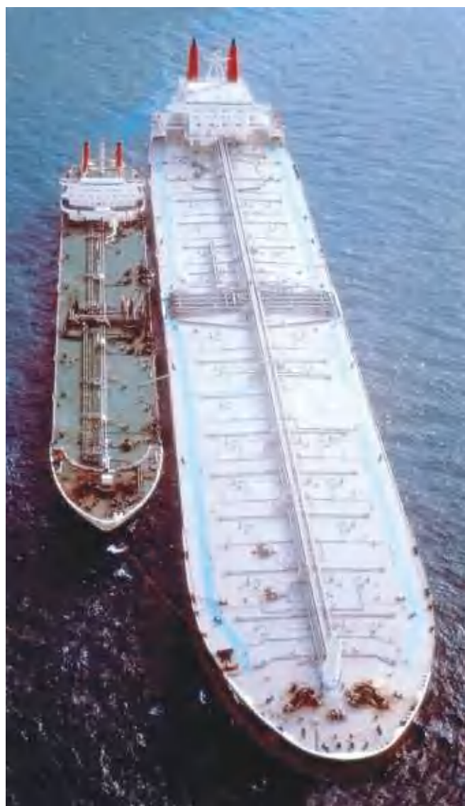
▲ The 553,662dwt Batillus (1,359ft by 206ft) in Lyme Bay, with the 71,917dwt Shell lightening tanker Drupa (800ft by 110ft) alongside. Batillus, scrapped only nine years after her completion by Chantiers de l'Atlantique in 1976, made 25 voyages between the Persian Gulf and northern Europe before being laid up in 1983 and sent to Kaohsiung, Taiwan for demolition in 1985. SOCIÉTÉ MARITIME SHELL FRANCAIS
