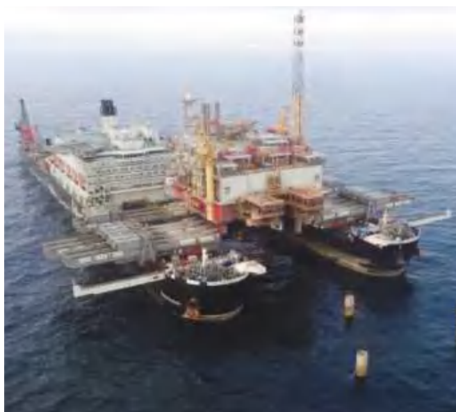
▲ A look at the world's largest ship, the 403,342gt Pioneer Spirit, just after it has clipped off and hoisted the 13,500-tonne topsides of the decommissioned Yme oil platform in the North Sea. PHOTO COURTESY OF ALLSEAS
