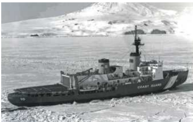
▲ Normally operating from her Pacific base at Seattle, Polar Star is used for exploration work at both poles, as well as in the Bering Sea. She is 399ft and is powered by three gas turbines, with three diesel engines for added propulsion.
