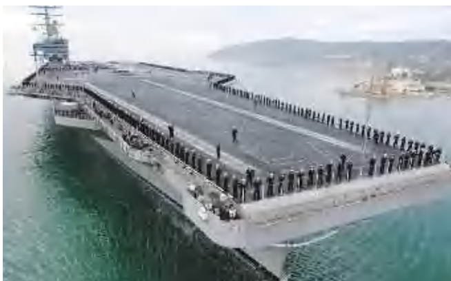
▲ USS Ronald Reagan (CVN-76), a Nimitz-class nuclear-powered aircraft carrier measuring 1,092ft (332.8m) by 252ft (76.8m) and displacing 101,400 long tons is the fastest of the big ships, with two Westinghouse A4W nuclear reactors powering four steam turbines of a combined 260,000shp (194 MW) to give a maximum speed of better than 30 knots. US NAVY
