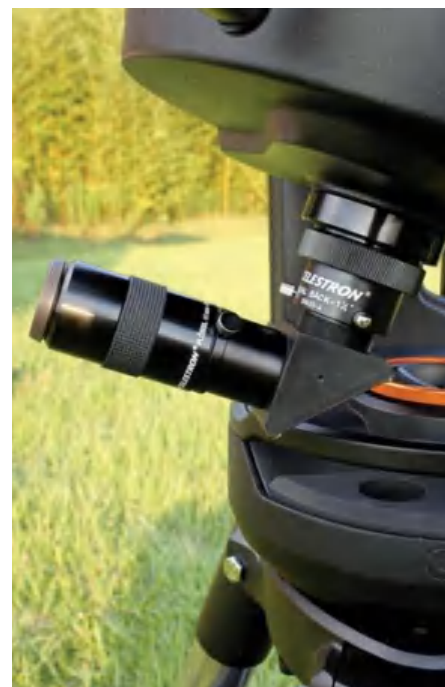
▲ As supplied, the NexStar Evolution 9.25 telescope in proper balance can only point about 70° up before its star diagonal hits the drive base. Adding a tube weight to the rear cell can alleviate the issue.
