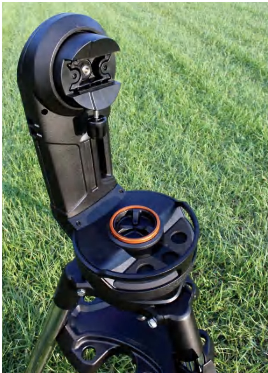
▲ Like most Celestron NexStar telescopes, the 9.25 is attached to the fork arm via a convenient Vixen-style dovetail system that allows users to remove or re-balance the OTA, though attaching the tube can be challenging due to the dovetail’s position on the side of the tube.
