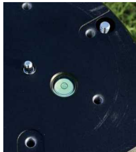
▲ The Evolution tripod includes a handy bubble level to quickly level the tripod before attaching the fork mount. A central pin helps to center the fork base.
