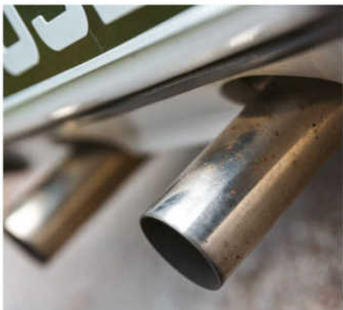
Left ST-style twin exit exhausts required Colin to modify the 3.2's rear valance to fit
