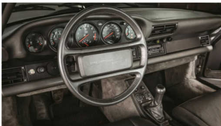
Above The 959 had the 911's iconic five dials, but the far right VDO clock was reserved for depicting torque split
