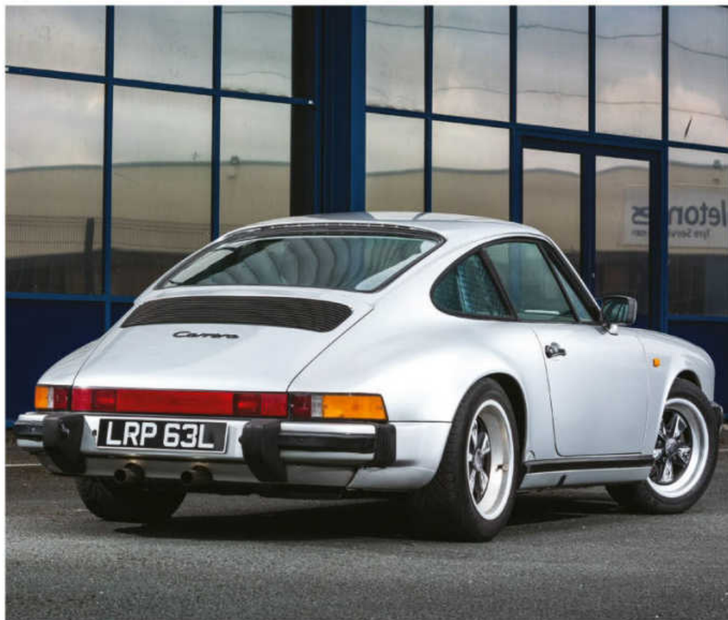
Left ST-style twin exit exhausts required Colin to modify the 3.2's rear valance to fit
