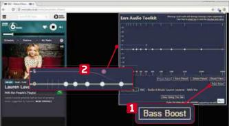
For a quick and simple fix, try clicking the Bass Boost button. 1 This increases the lower frequency levels, which you can see represented by the purple line on the left-hand side of the graph. 2 If you're listening through earbuds, this setting can give you a significantly richer sound.
