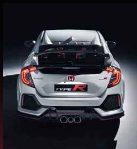
Above: the old Type R's four exhaust tips have become three, moved to the middle of the rear valance (very 458...)
