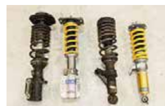
Above: old and new spring and damper units side by side. Below: new adjustable top mounts. Bottom: getting the geometry just-so
