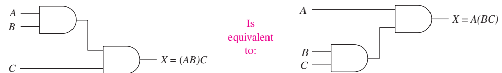
Figure 5-11 Using the associative law of multiplication to rearrange the grouping of AND gates.
