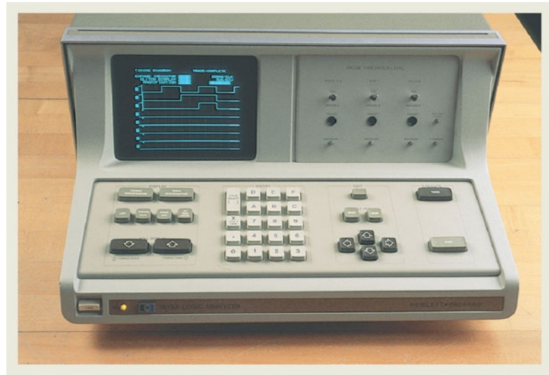
Figure 3-10 Timing analysis of an AND gate: (a) waveform sketch; (b) actual logic analyzer display.
