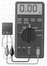
(b) Forward- and reverse-bias tests for a shorted junction give the same 0 V reading. If the junction is resistive, the reading is less than 2.6 V.
