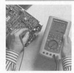
In this system application, we are focusing on the two audio amplifier boards in an FM stereo receiver. Both boards are identical except one is for the left channel sound and the other is for the right channel sound. This circuit is a good example of a mixed use of an integrated circuit and discrete components.
