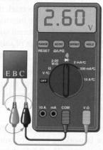
(a) Forward-bias test and reversebias test give the same reading (2.60 V is typical) for an open BC junction.
