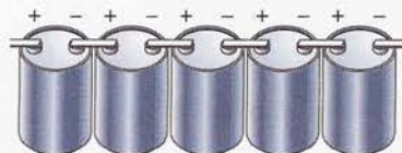
(a) Series-connected battery
