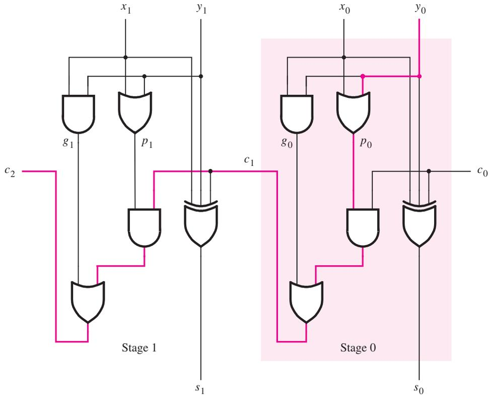
**Figure 3.14** A ripple-carry adder based on expression 3.3.
