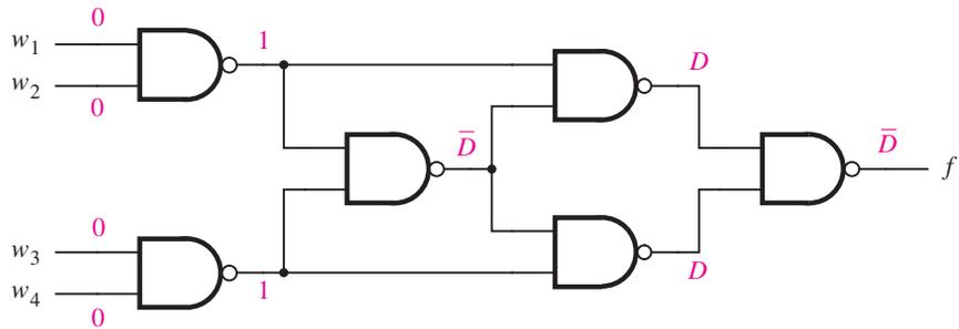
(c) Detection of  $g/1$  fault**Figure 11.4** Detection of faults.
