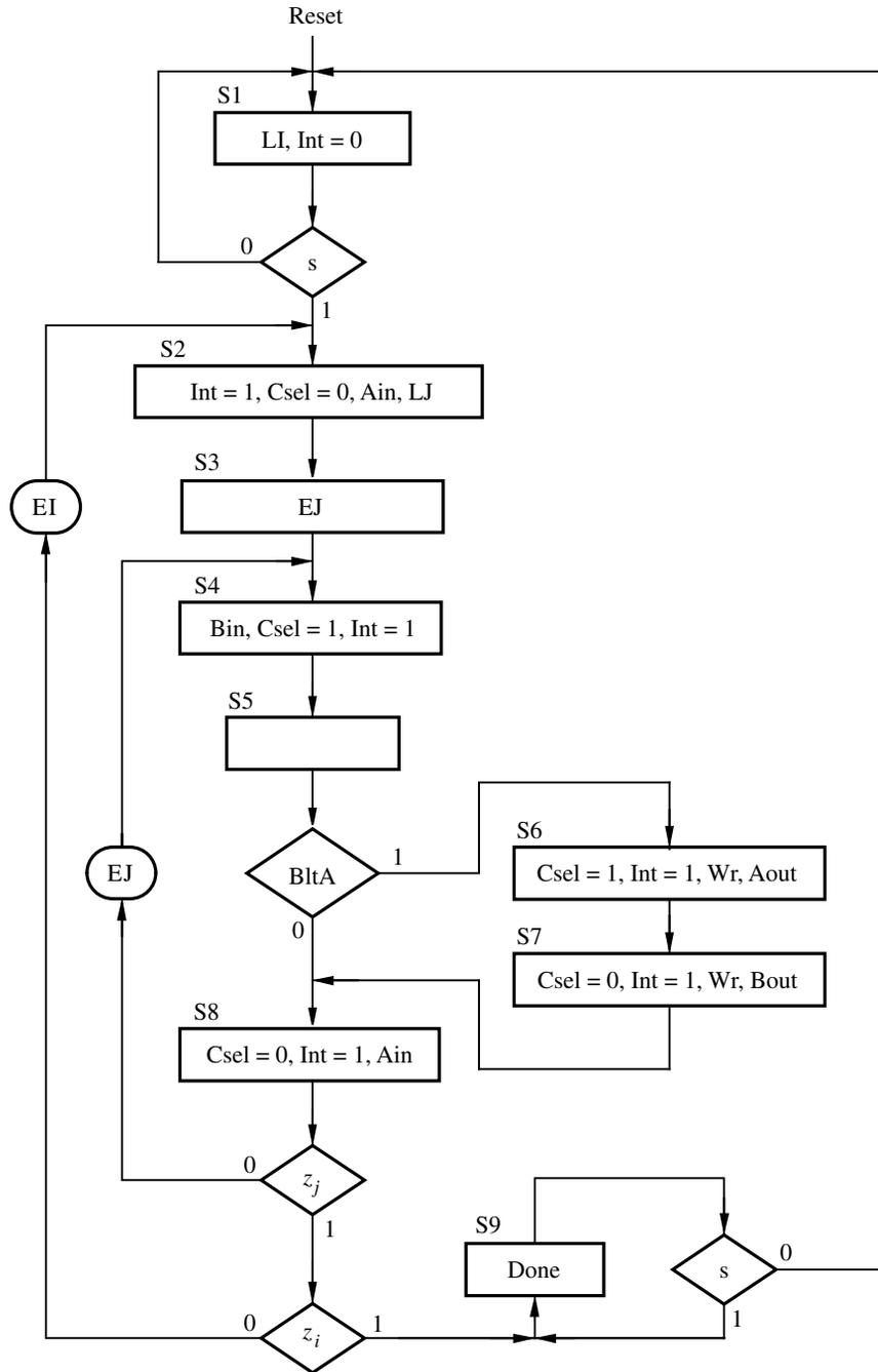
**Figure 7.44** ASM chart for the control circuit.
