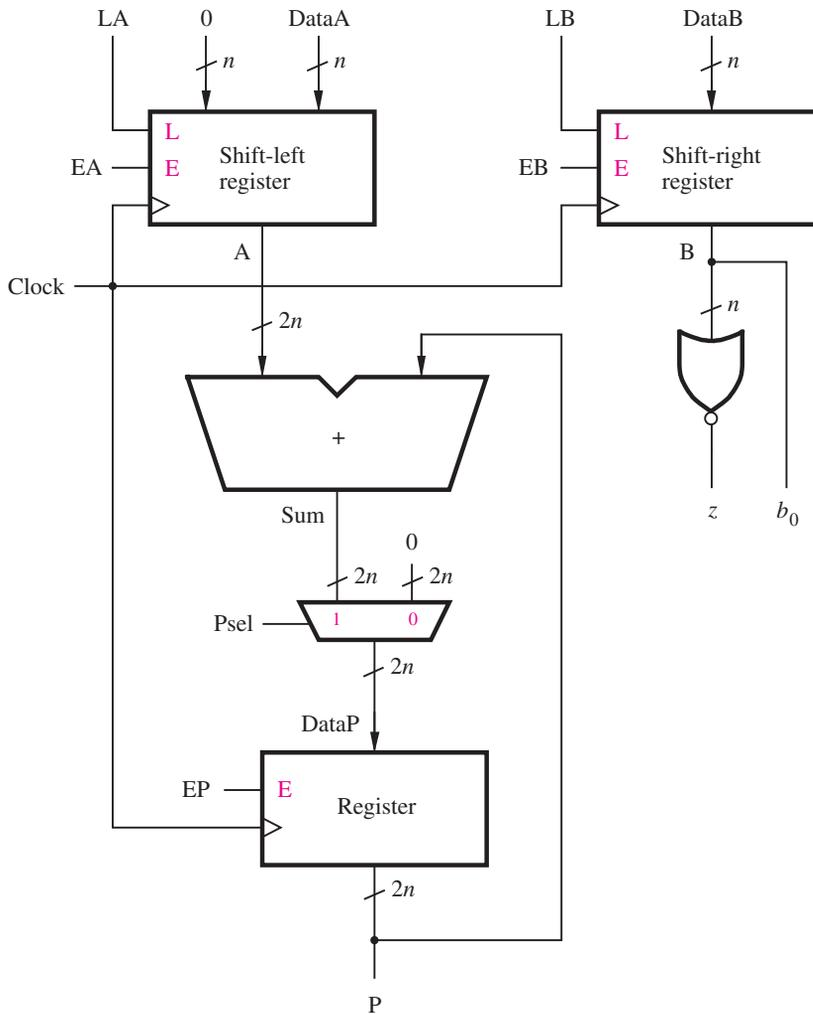
**Figure 7.24** Datapath circuit for the multiplier.
