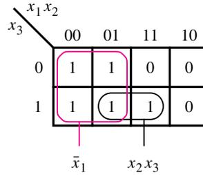
**Figure 2.56** Three-variable function  $f(x_1, x_2, x_3) = \sum m(0, 1, 2, 3, 7)$ .
