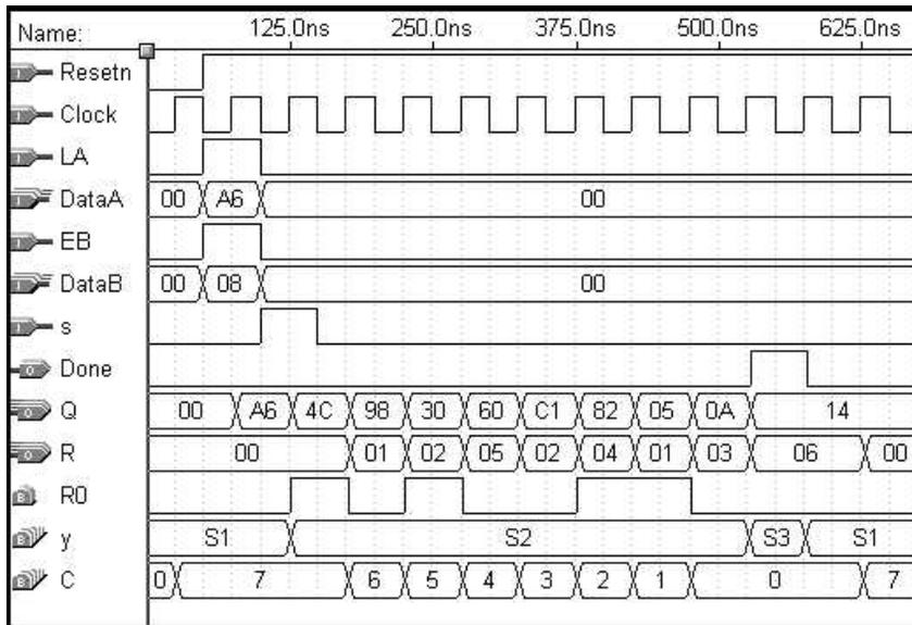
**Figure 7.36** Simulation results for the divider circuit.
