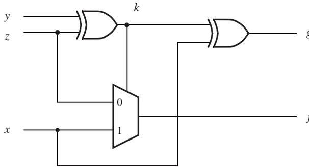
**Figure 2.70** The logic circuit for Example 2.29.
