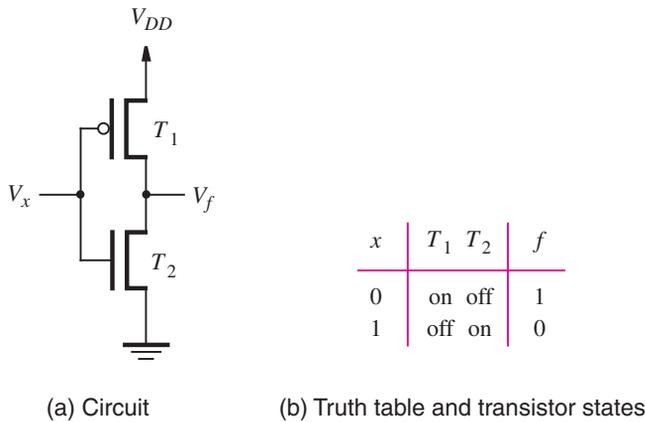
**Figure B.12** CMOS realization of a NOT gate.
