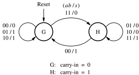
**Figure 6.40** State diagram for the serial adder FSM.
