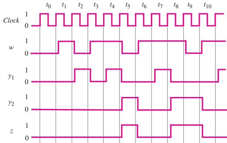
**Figure 6.9** Timing diagram for the circuit in Figure 6.8.
