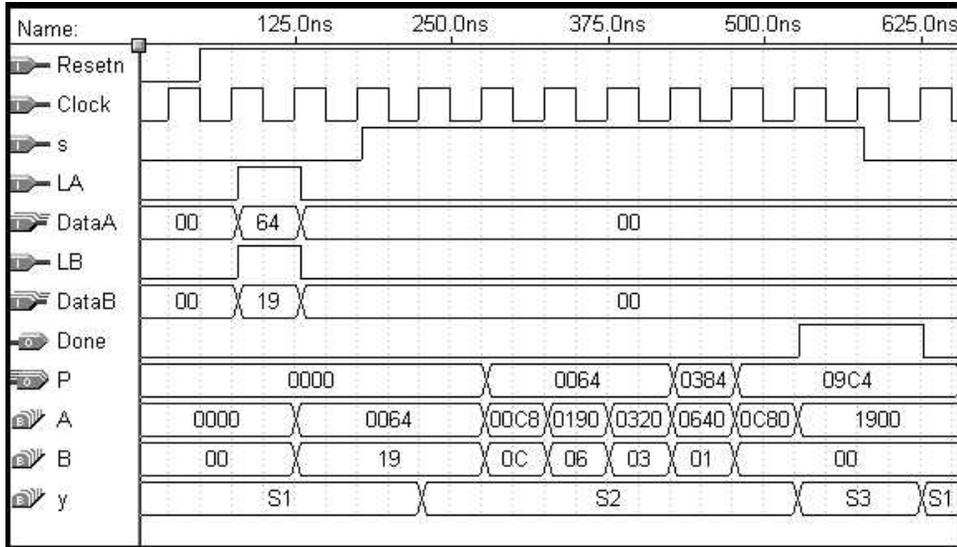
**Figure 7.27** Simulation results for the multiplier circuit.
