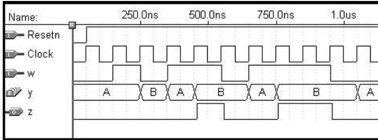
**Figure 6.37** Simulation results for the Mealy machine.
