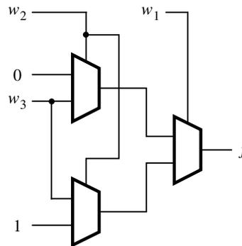
**Figure 4.12** The circuit synthesized in Example 4.6.
