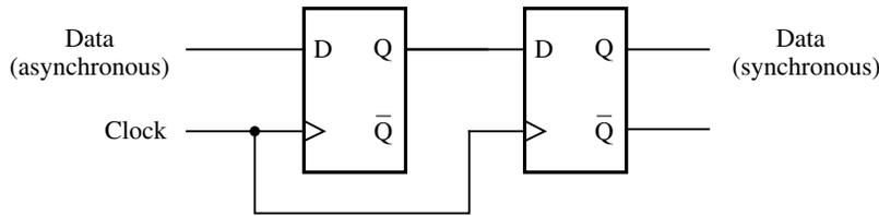
**Figure 7.50** Asynchronous inputs.
