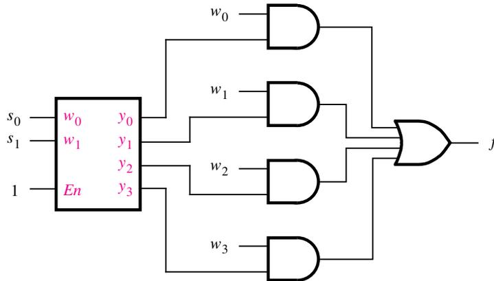
**Figure 4.17** A 4-to-1 multiplexer built using a decoder.
