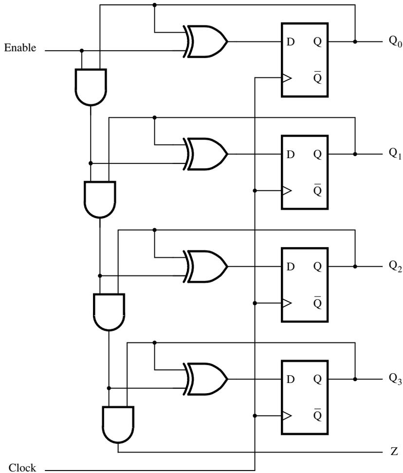
**Figure 5.23** A four-bit counter with D flip-flops.
