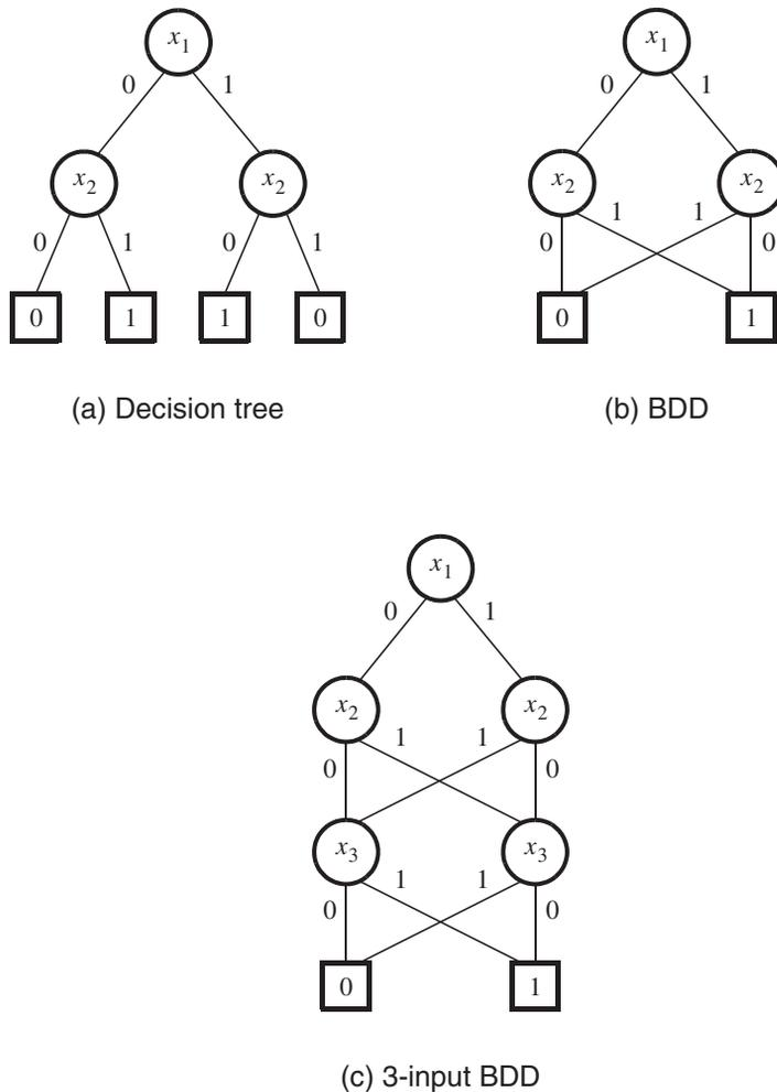
**Figure 8.21** Derivation of BDDs for XOR functions.
