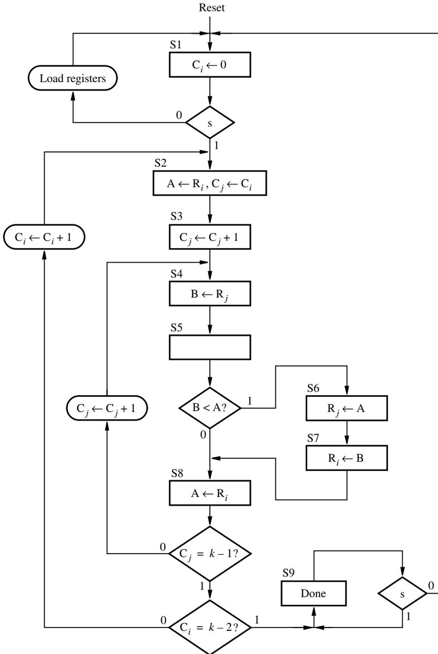
**Figure 7.41** ASM chart for the sort operation.
