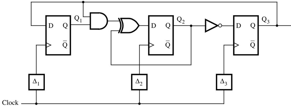
**Figure 5.76** A circuit with clock skews.
