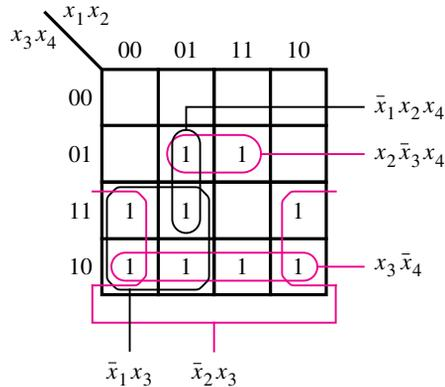
**Figure 2.57** Four-variable function  $f(x_1, \dots, x_4) = \sum m(2, 3, 5, 6, 7, 10, 11, 13, 14)$ .
