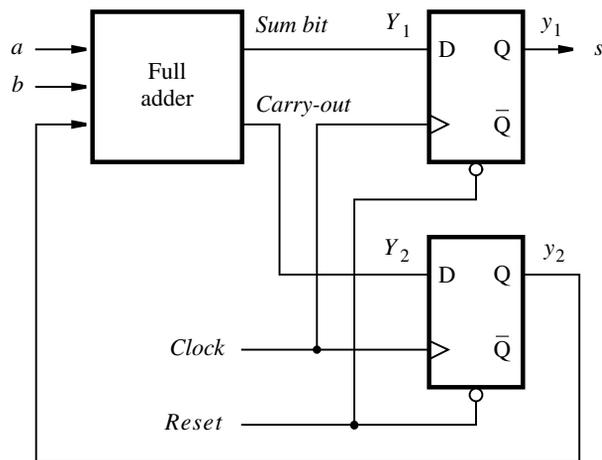
**Figure 6.47** Circuit for the Moore-type serial adder FSM.
