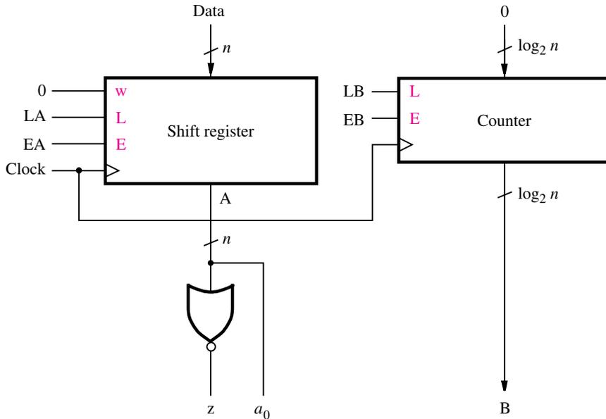
**Figure 7.18** Datapath for the ASM chart in Figure 7.17.
