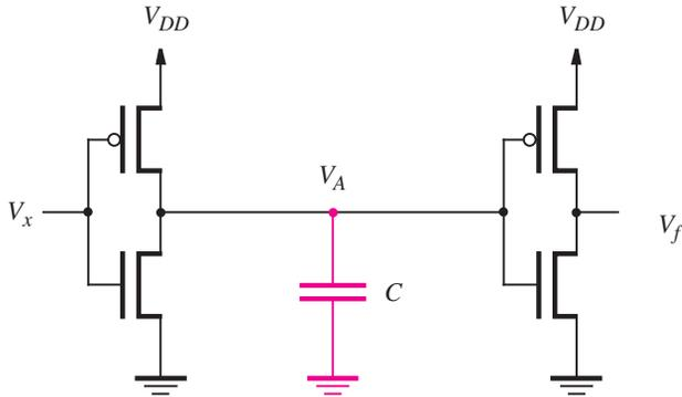
(b) The capacitive load at node  $A$ **Figure B.47** Parasitic capacitance in integrated circuits.
