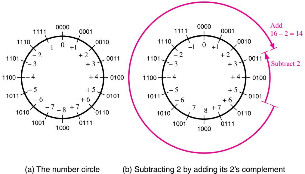
**Figure 3.11** Graphical interpretation of four-bit 2's complement numbers.
