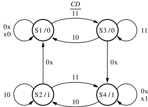
**Figure 9.7** State diagram for the master-slave D flip-flop.
