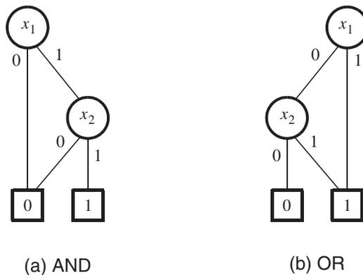
**Figure 8.20** BDDs for the AND and OR functions.
