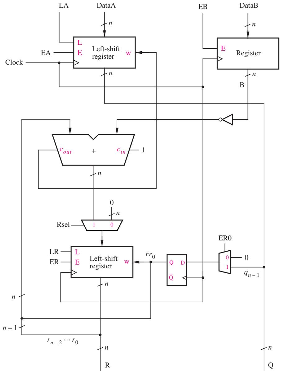
**Figure 7.34** Datapath circuit for the enhanced divider.
