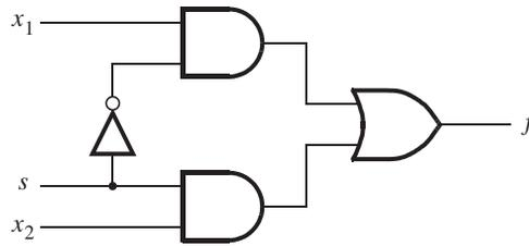
**Figure 2.36** The logic circuit for a multiplexer.
