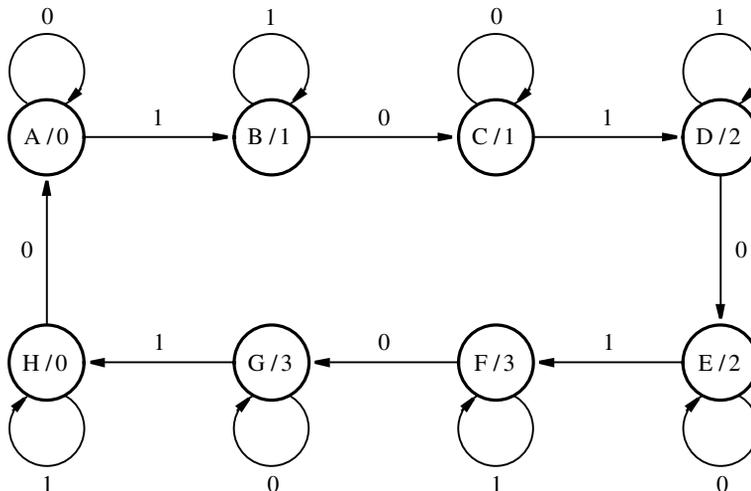
**Figure 9.17** State diagram for a modulo-4 counter.
