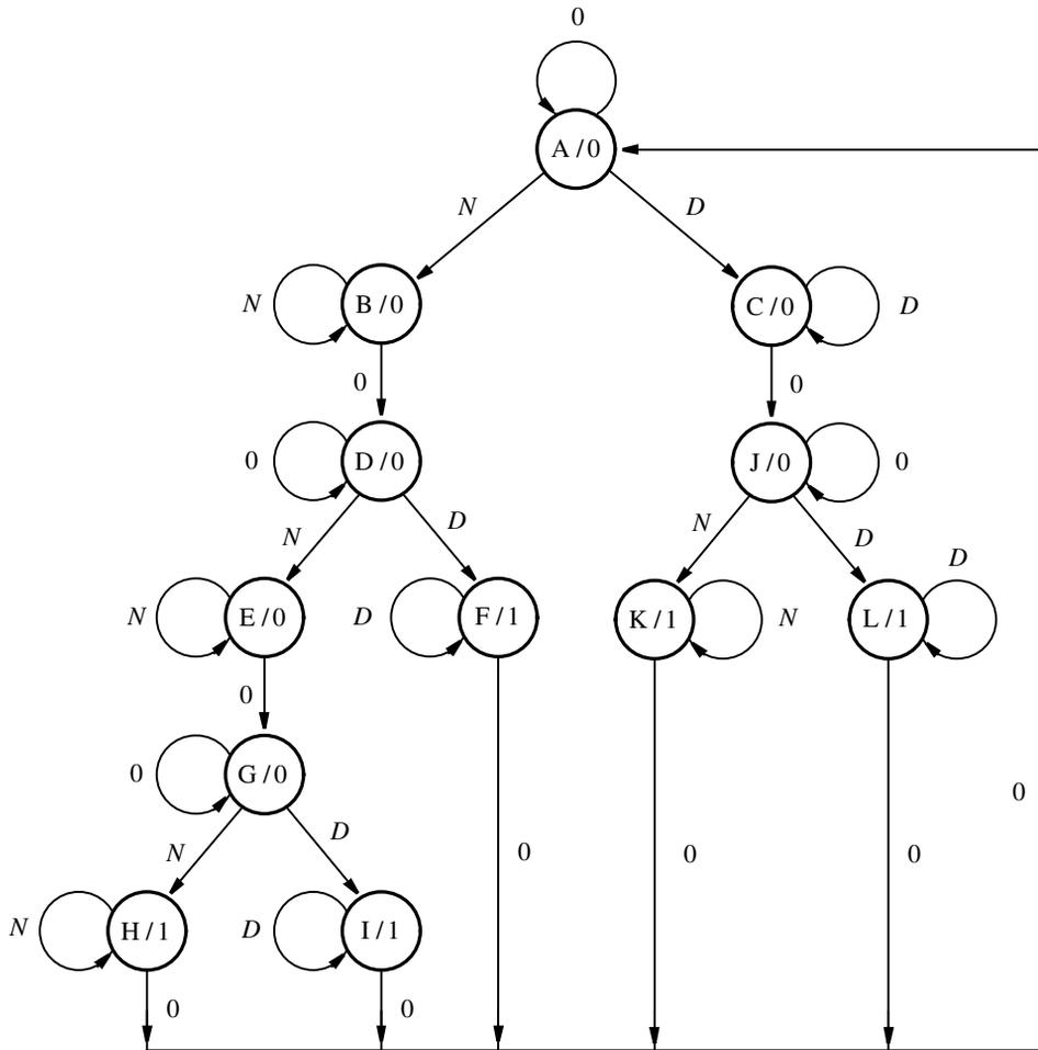
**Figure 9.67** Initial state diagram for the vending-machine controller.
