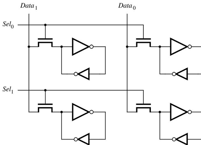
**Figure B.65** A  $2 \times 2$  array of SRAM cells.
