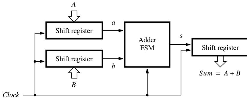
**Figure 6.39** Block diagram for the serial adder.
