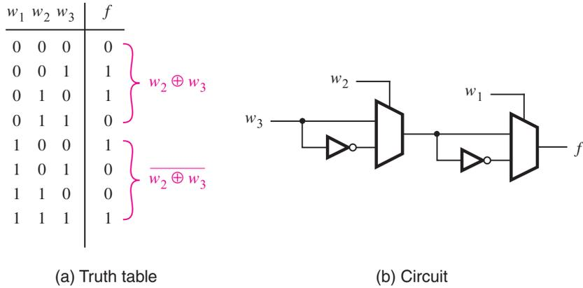
**Figure 4.8** Three-input XOR implemented with 2-to-1 multiplexers.
