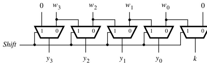
**Figure 4.50** A shifter circuit.
