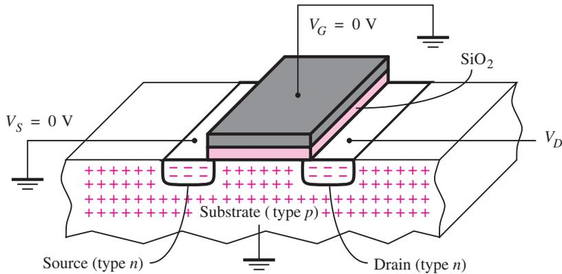
(a) When  $V_{GS} = 0\text{ V}$ , the transistor is off
