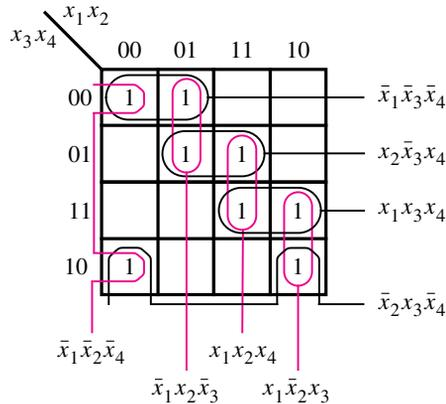
**Figure 2.59** The function  $f(x_1, \dots, x_4) = \sum m(0, 2, 4, 5, 10, 11, 13, 15)$ .
