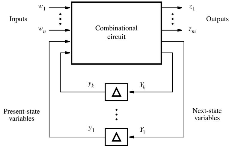
**Figure 6.85** The general model for a sequential circuit.
