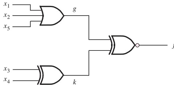
**Figure 8.8** Decomposition for Example 8.3.
