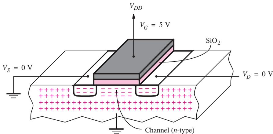
(b) When  $V_{GS} = 5\text{ V}$ , the transistor is on**Figure B.43** Physical structure of an NMOS transistor.
