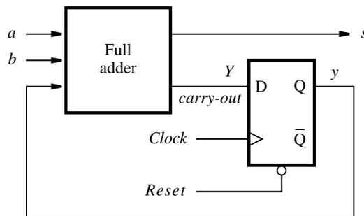
**Figure 6.43** Circuit for the adder FSM in Figure 6.39.
