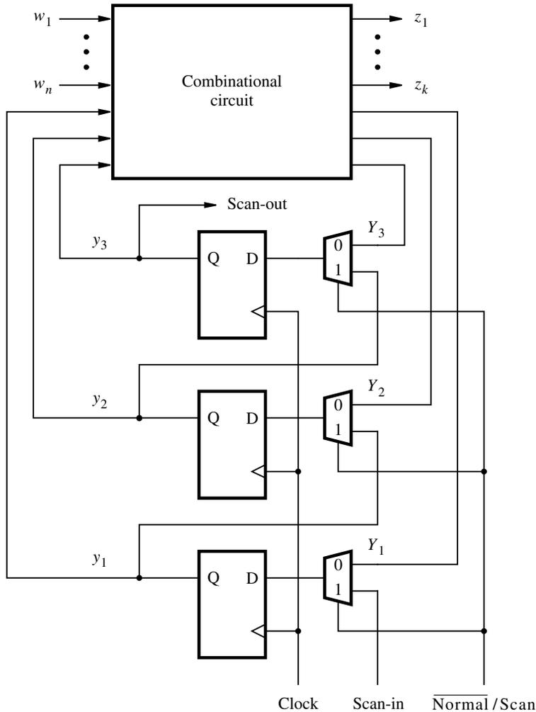
**Figure 11.11** Scan-path arrangement.
