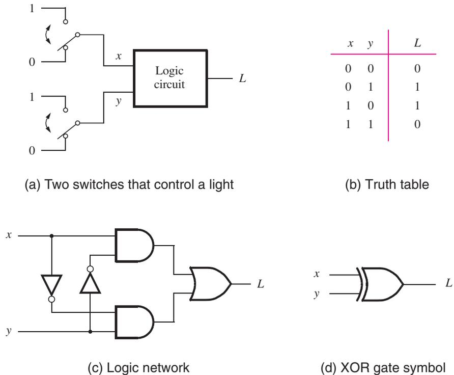
**Figure 2.11** An example of a logic circuit.
