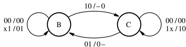
**Figure 9.24** Mealy model for the arbiter FSM.
