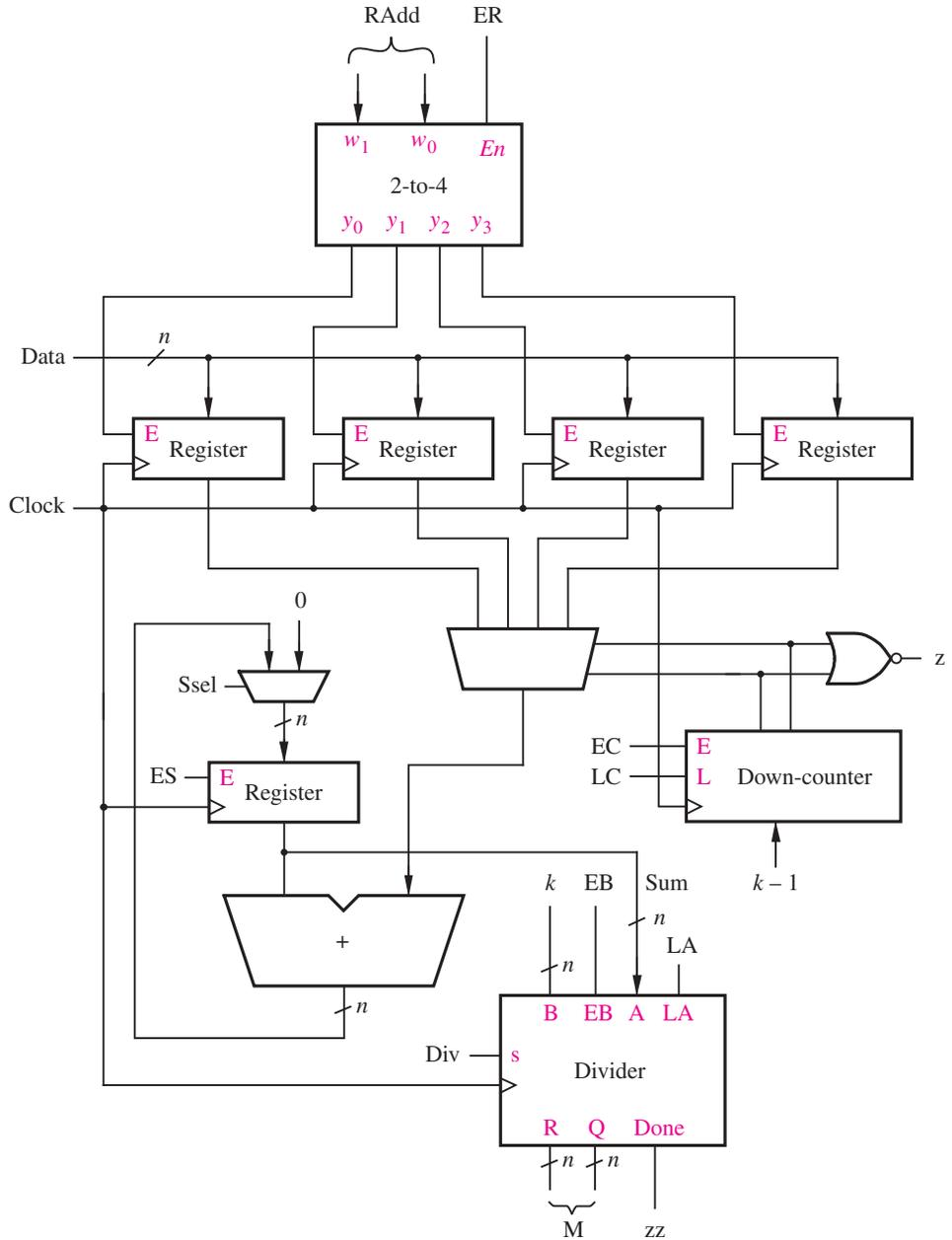
**Figure 7.38** Datapath circuit for the mean operation.
