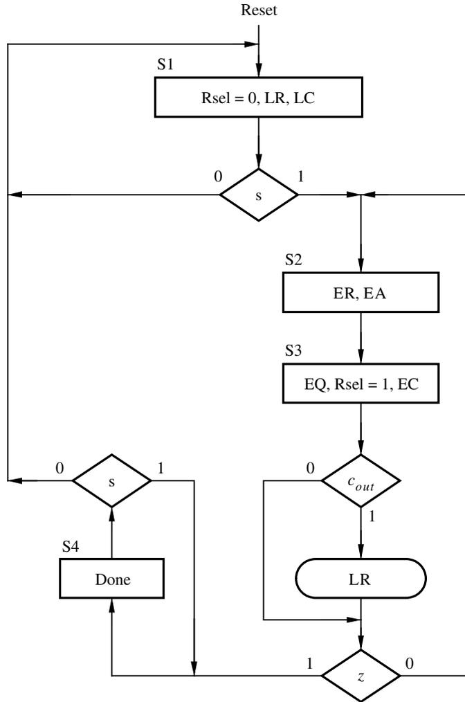
**Figure 7.31** ASM chart for the divider control circuit.
