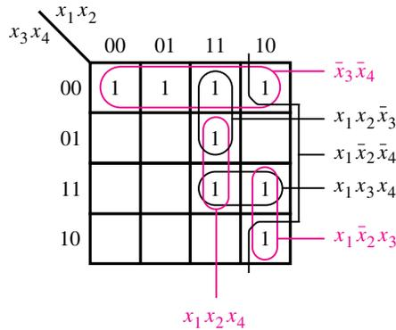
**Figure 2.58** The function  $f(x_1, \dots, x_4) = \sum m(0, 4, 8, 10, 11, 12, 13, 15)$ .
