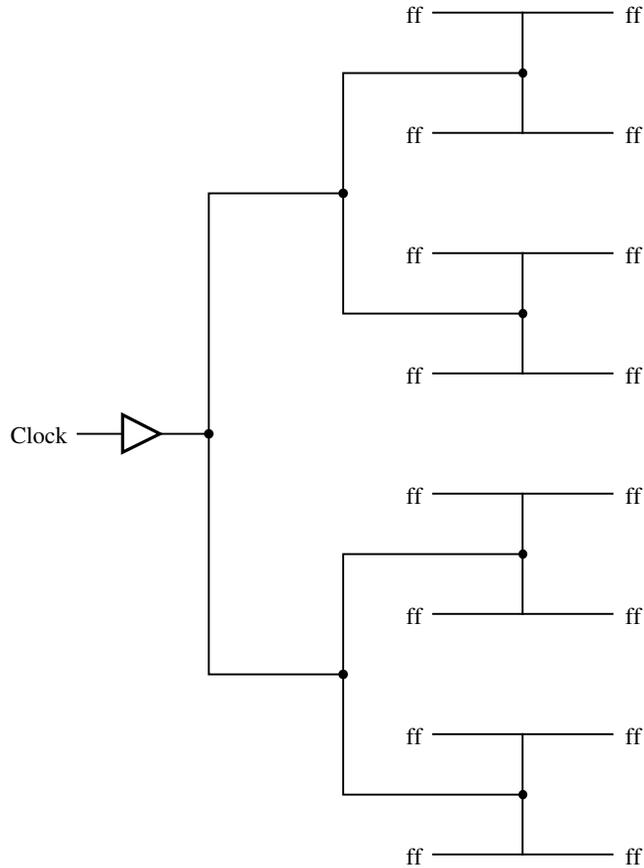
**Figure 7.47** An H tree clock distribution network.
