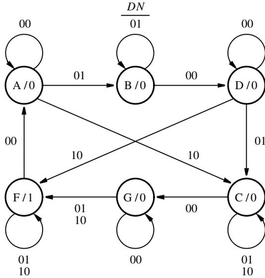
**Figure 9.72** State diagram for the vending-machine controller.
