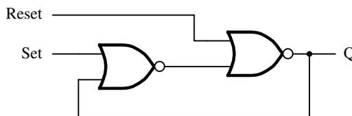
**Figure 5.3** A memory element with NOR gates.
