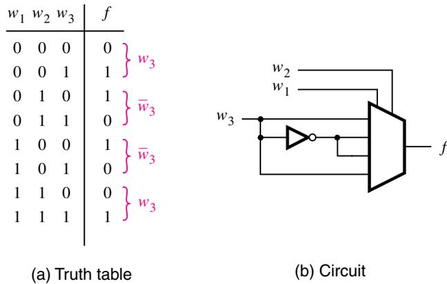
**Figure 4.9** Three-input XOR implemented with a 4-to-1 multiplexer.
