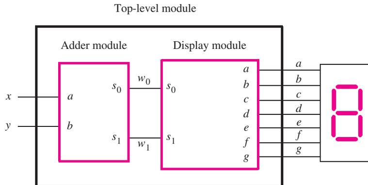
**Figure 2.44** A logic circuit with two modules.
