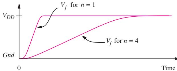
(c) Propagation times for different values of  $n$ **Figure B.59** The effect of fan-out on propagation delay.
