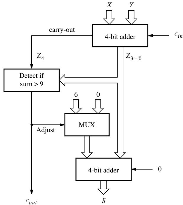
**Figure 3.39** Block diagram for a one-digit BCD adder.
