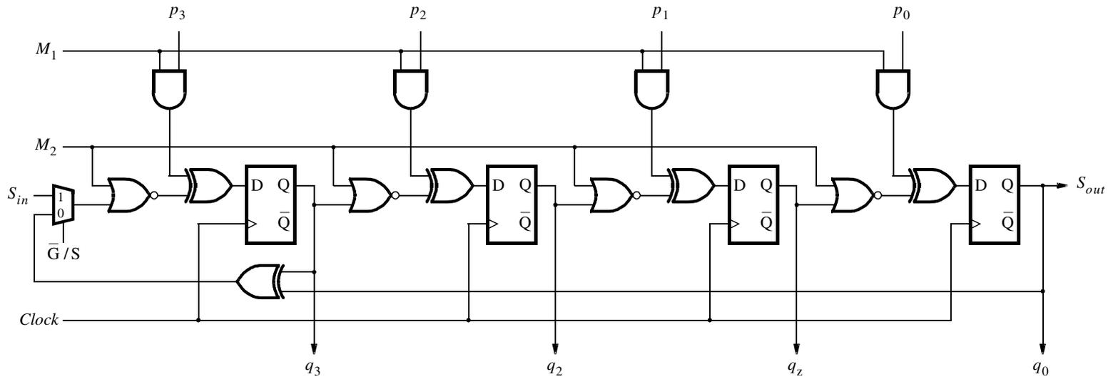
**Figure 11.18** A four-bit built-in logic block observer (BILBO).
