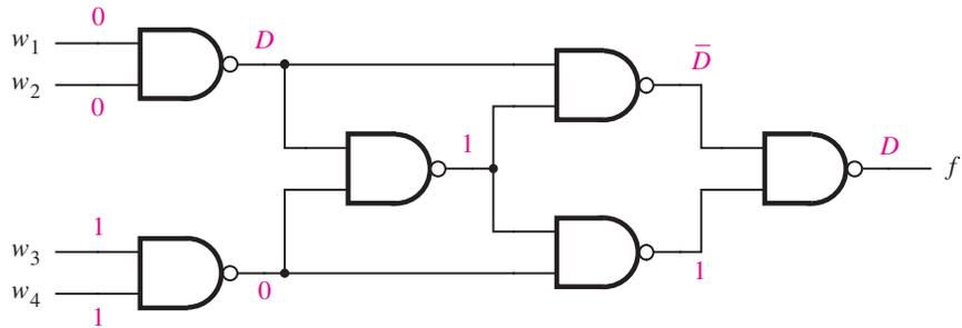
(b) Detection of  $b/0$  fault
