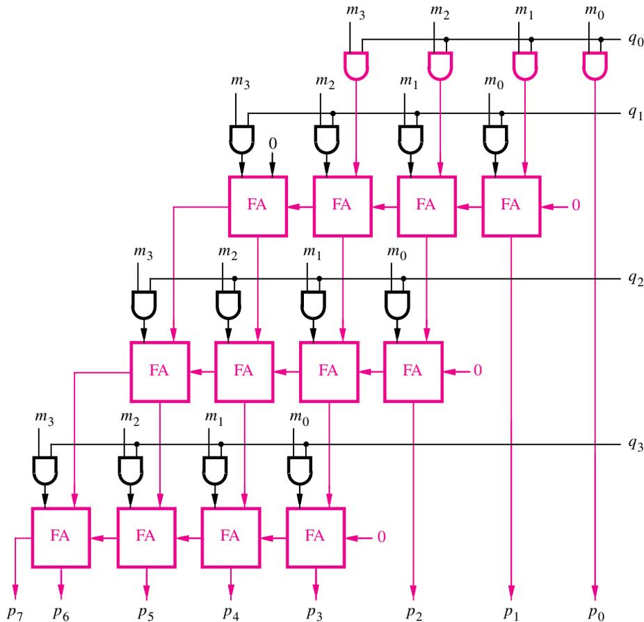
**Figure 3.35** A  $4 \times 4$  multiplier circuit.
