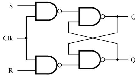
**Figure 5.6** Gated SR latch with NAND gates.
