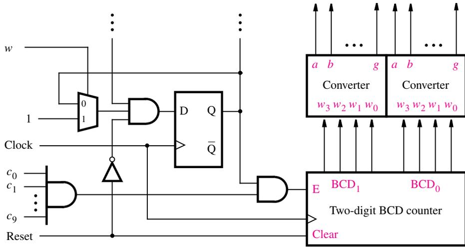
**Figure 5.69** A modified version of the reaction-timer circuit.
