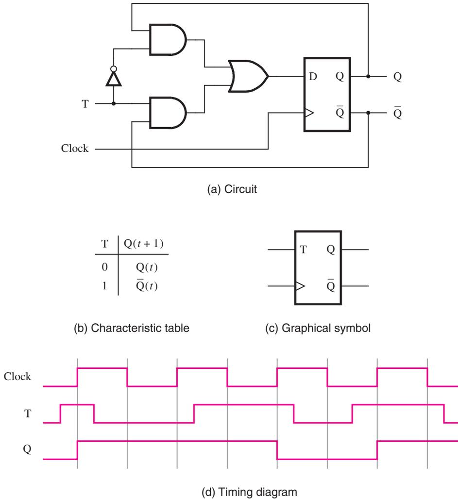
**Figure 5.15** T flip-flop.
