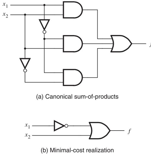
**Figure 2.20** Two implementations of the function in Figure 2.19.
