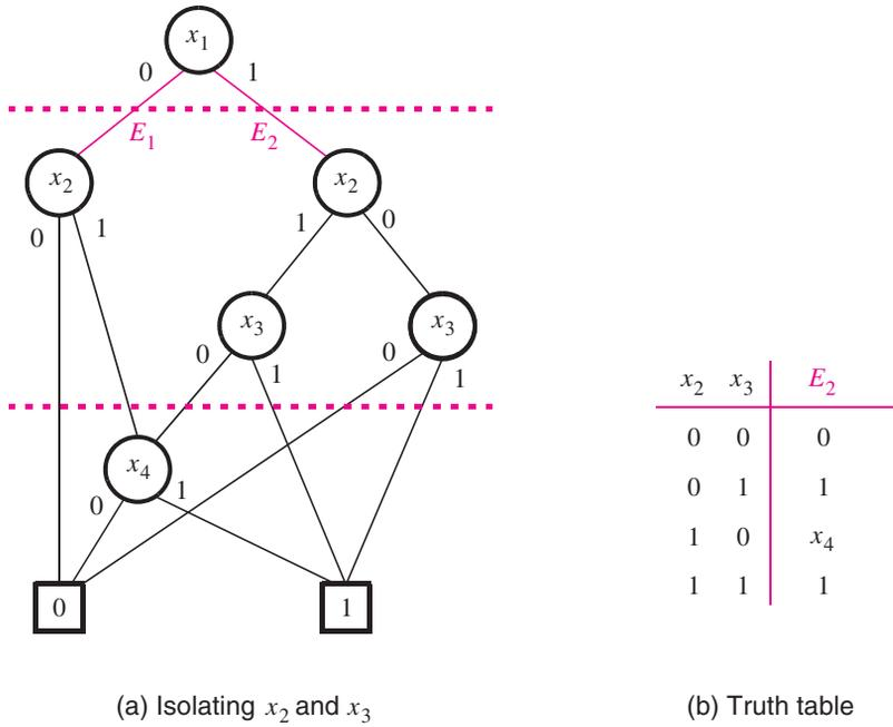
**Figure 8.36** Reordering the BDD in Figure 8.35.
