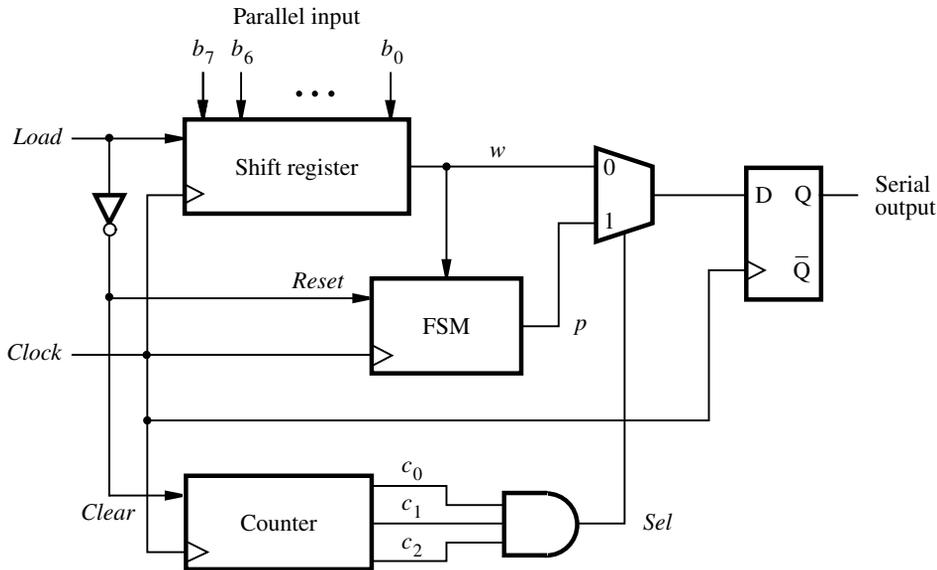
**Figure 6.97** Parallel-to-serial converter.
