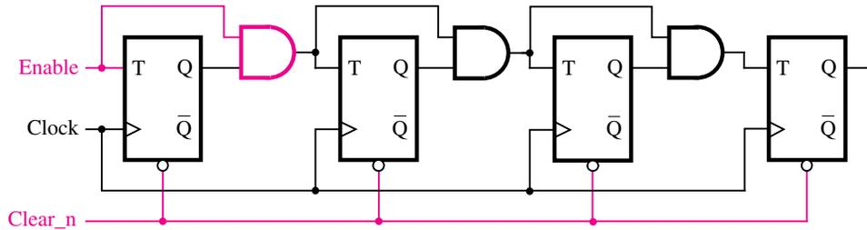
**Figure 5.22** Inclusion of Enable and Clear capability.
