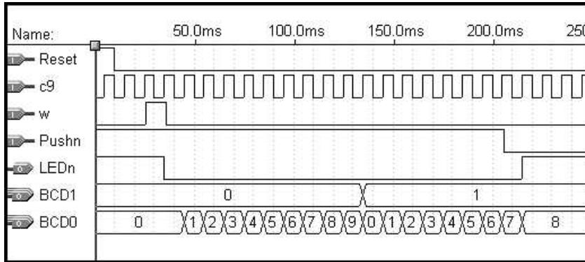
**Figure 5.65** Simulation of the reaction timer circuit.
