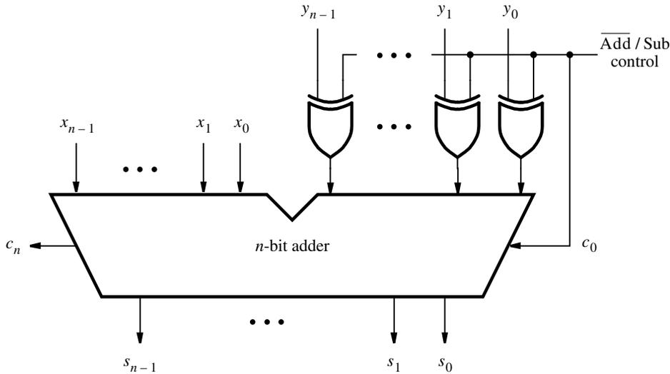
**Figure 3.12** Adder/subtractor unit.
