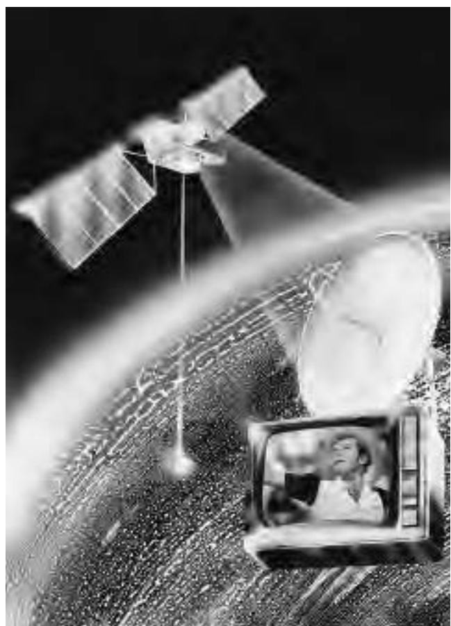
An artist's rendering of a direct broadcast satellite (DBS) and the small (typically less than 0.5-meter-diameter) rooftop satellite dish that is equipped to decode DBS transmissions, bringing numerous television channels and other signals into individual households ( Artist's rendering courtesy of CNES )
