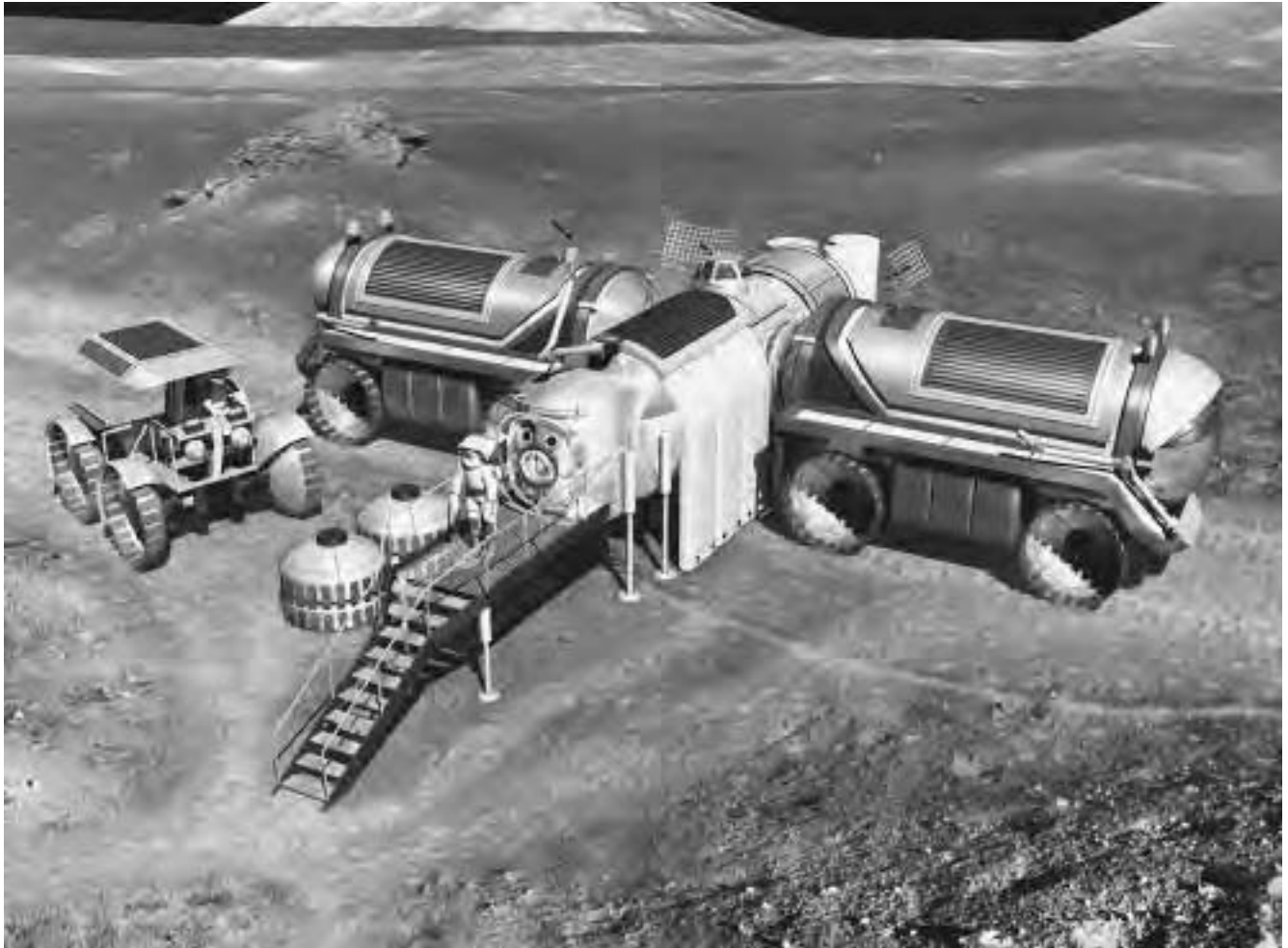
This is an artist's conception of a lunar habitat being assembled out of components delivered to the Moon's surface by a series of automated cargo flights ca. 2020. Pressurized rovers, logistics modules, and a space suit maintenance and storage module combine to provide the living and working quarters for the lunar astronauts. (Courtesy of NASA; artist, John Frassanito and Associates [1993])
