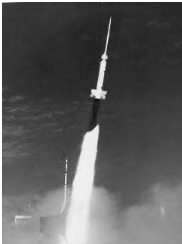
A Nike-Apache sounding rocket blasts off from NASA's Wallops Flight Facility, Wallops Island, Virginia, in 1965. In its seven-minute, ballistic trajectory flight over the Atlantic Ocean, this rocket's scientific payload, designed to make measurements within the ionosphere, reached a maximum altitude of approximately 180 kilometers. (Courtesy of NASA)
