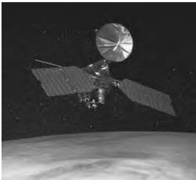
This artist's rendering shows NASA's Mars Reconnaissance Orbiter spacecraft taking extremely high-resolution images of the planet's surface and using its sounder to investigate scientifically interesting areas for possible subsurface water ca. 2006. (Artist's rendering courtesy of NASA/JPL)
