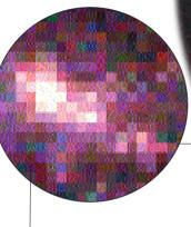
A magnified CCD image breaks up into colored squares, or pixels, showing that it is a digital image.
