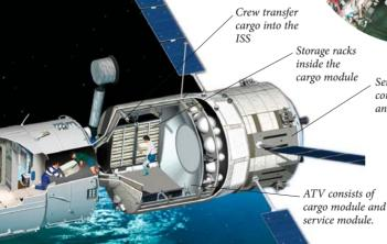
Service module controls four engines and 28 thrusters.
