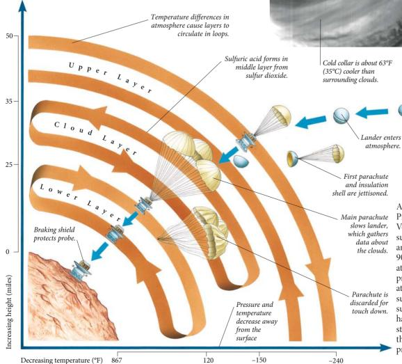
ATMOSPHERIC STUDY Probes sent to fly through Venus's atmosphere have to survive the corrosive clouds and the high pressure, which is 90 times greater than the Earth's at surface level. A number of probes have entered the atmosphere, and some have succeeded in reaching the surface. Between them, they have revealed the atmosphere's structure and composition, and the range of temperatures and pressures within it.
