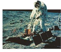
APOLLO SCIENTIFIC EXPERIMENTS The astronauts left behind experiments, plus equipment to send the results back to Earth. They measured moonquakes (movements in the lunar crust), the soil temperature, the
