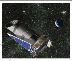
Telescope has a 3-ft-(0.95-m-) wide mirror and always points in the same direction.
