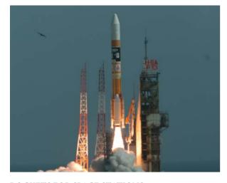
H-IIA has been Japan's primary large-scale launch vehicle since 2001. The number of strap-on boosters depends on the size and weight of the satellite it launches.
