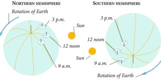
The shadow on a sundial moves clockwise as the Earth rotates in the northern hemisphere.
