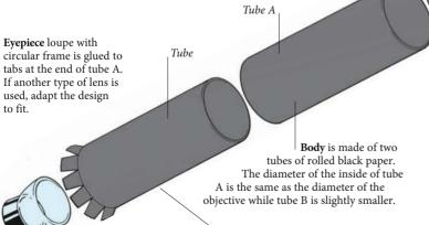
**Objective** is glued to one side of the plain black ring. The other side of the ring is glued to the tabbed ring. Fold the tabs toward the objective and slide the assembly 1 in (2.5 cm) inside tube A. Glue tabs to the inside of the tube so that ends are level with the tube's end.
