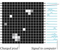
Pixels in a CCD are silicon squares separated by thin insulating walls. Light hitting a pixel ejects negatively charged electrons from the silicon, building up a positive charge.
