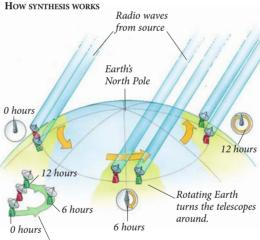
View from space: the green telescope appears to make a half-circle around the red telescope over 12 hours. Without moving the telescopes, this method has filled in part of a much larger "dish."
