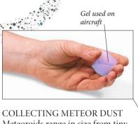
Meteoroids range in size from tiny dust particles of one-millionth of a gram to 1-ton space rocks. For the past 20 years, scientists have been collecting and studying the smaller particles. Aircraft with gel-covered panels cruise at altitudes of about 12 miles (20 km). When the fastmoving particles collide with the gel they stick to it and can be studied later in the laboratory.
