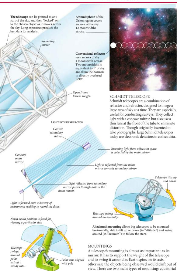
**Equatorial mounting** has axis of the mount pointing at the celestial pole (north or south, depending on the hemisphere). The telescope swivels around the axis to follow the stars as they circle the pole.
