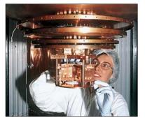
SERVICING THE CRESST WIMP DETECTOR IN ITALY
