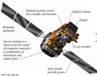
Integral was launched in 2002 and can observe gamma rays, X-rays, and visible light from objects simultaneously. It carries four main instruments. Two gamma-ray instruments make images and analyze the range of energy covered by the radiation. An X-ray monitor and optical camera help to identify gamma-ray sources. Integral is in an elongated elliptical orbit around Earth, avoiding the planet's radiation belts, which would interfere with its measurements.
