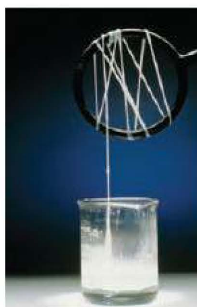
Figure 14.2 The synthetic fibre, nylon is made by the condensation polymerisation of amine-containing molecules and carboxylic acid-containing molecules to form long chains (polymers). Nylon is used to make fabrics, and also ropes and some medical prosthetics.
