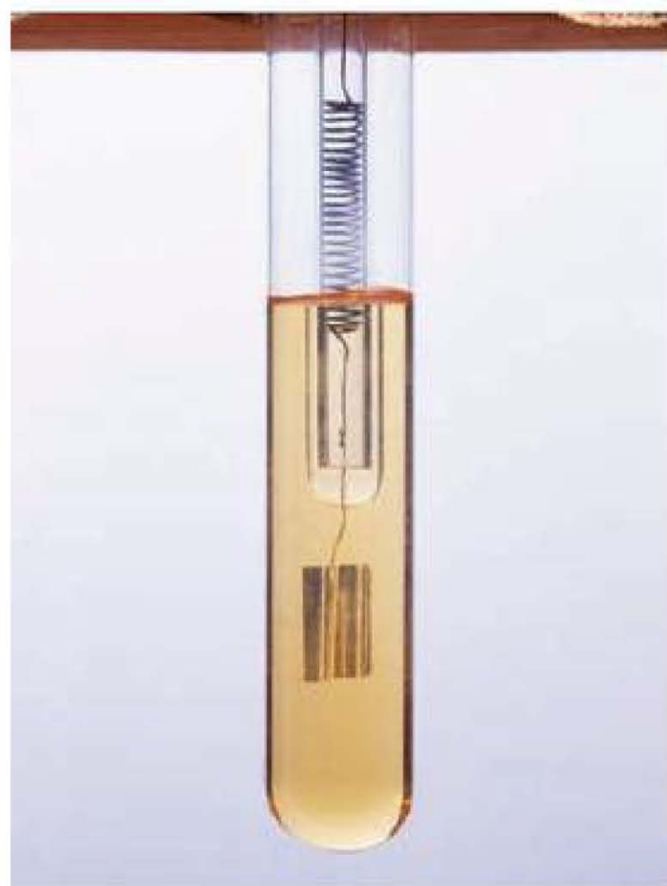
Figure 5.4 A platinum electrode (square, lower centre) in a solution of iron(II) and iron(III) ions. The iron(III) ions are being reduced to iron(II) ions, gaining an electron in the process. The electron movements are powered by the oxidation of hydrogen in the smaller tube seen inside the larger tube. Hydrogen gas is adsorbed onto the platinum coil and loses two electrons to form two hydrogen ions in the surrounding water. A platinum-hydrogen electrode is the standard used to measure redox potentials of ions. In this case the iron(III) to iron(II) redox potential is +0.77V.
