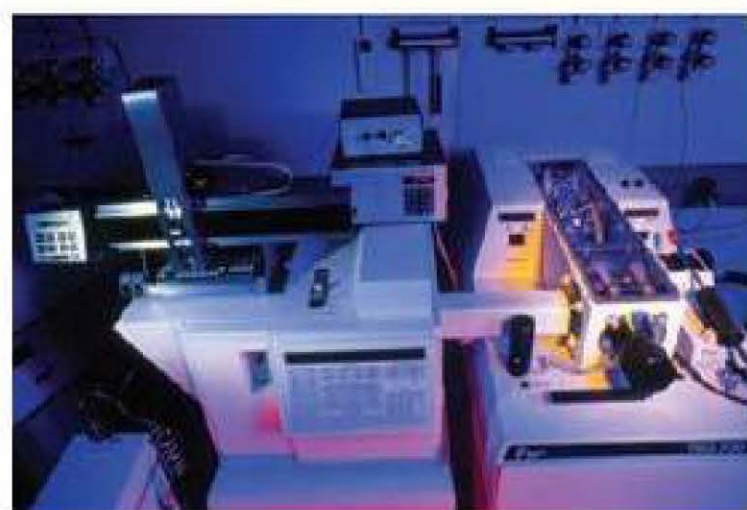
Figure 15.5 A gas chromatography machine (left) connected to a mass spectrometer (right) in a forensic laboratory. This equipment is sensitive enough to detect minute quantities of illegal drugs in the hair of a suspect – weeks after any drugs were taken.
