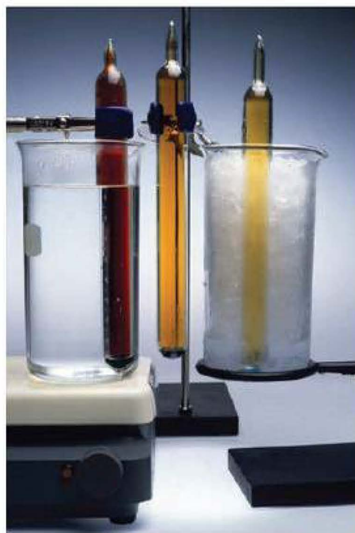
Figure 4.1 The equilibrium between \text{NO}_2 and \text{N}_2\text{O}_4 is shown in cold and hot water baths. A change in temperature shifts the equilibrium between the two species. When more \text{NO}_2 is produced, the gas inside the tube becomes darker. The K_p value will change with temperature.
