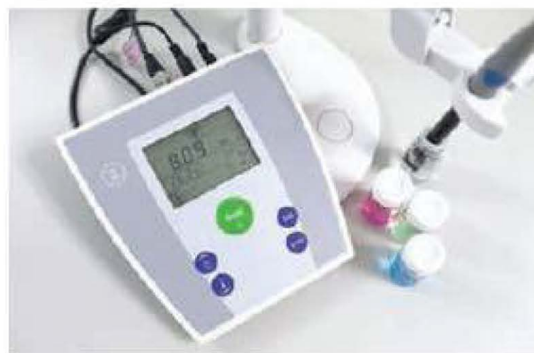
Figure 6.6 The pH of a solution can be accurately measured using a digital pH meter. The pH of this solution is 8.09.
