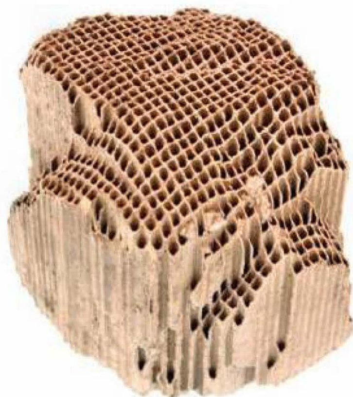
Figure 9.2 The catalyst found in a catalytic converter is usually platinum or rhodium plated onto a ceramic honeycomb structure. The honeycomb structure allows for a larger surface area for the reactant gases to undergo chemisorption on the surface of the catalysts.
