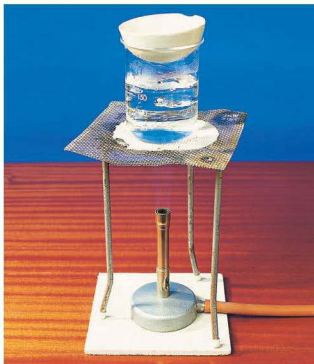
Figure 8.12 The solution of magnesium nitrate is concentrated by slow evaporation.
