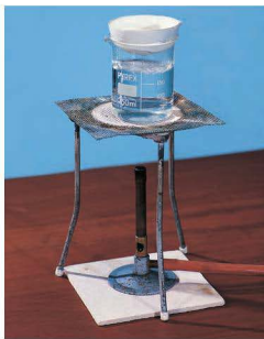
Figure 2.16 Apparatus used to slowly evaporate a solvent.
