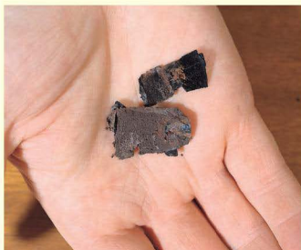
Figure 5.21 This plastic has been coated with copper by electrolysis.
