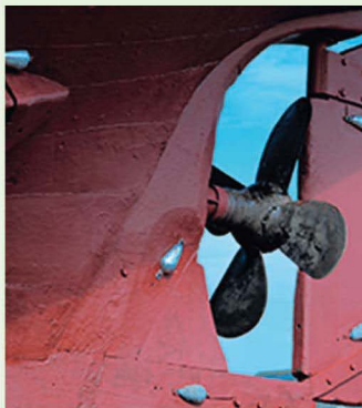
a Bars of zinc on the hull of a ship.
