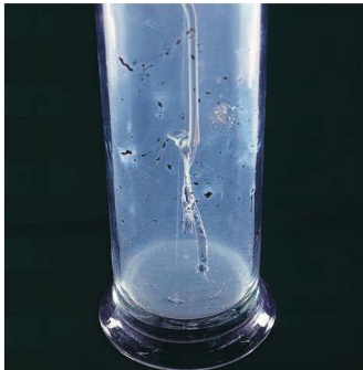
Figure 13.17 When magnesium burns in carbon dioxide gas, magnesium oxide (white) and carbon (black) are produced.
