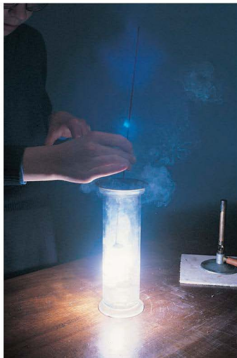
Figure 2.7 Magnesium burns brightly in oxygen to produce magnesium oxide.
