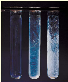
Figure 11.32 Evaporating pure water leaves no deposit, while temporary or permanent hard water leaves white deposits behind.
