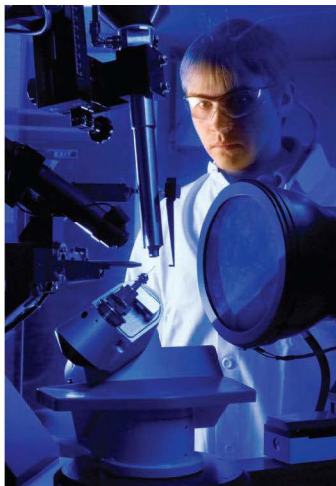
Figure 1.4 A modern X-ray crystallography instrument, used for studying crystal structure.
