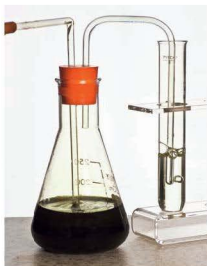
Figure 9.13 Iodine being displaced from potassium iodide solution as chlorine is bubbled through.
