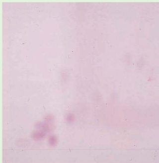
Figure 15.24 Amino acids can be separated and identified by TLC.
