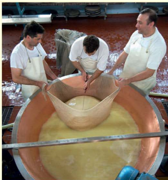
Figure 7.21 Cheese is separated into curds and whey by the addition of bacteria. The liquid, whey, is separated from the curds which are then pressed.
