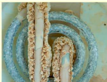
a The deposit in kettles ('furring') is caused by calcium carbonate from hard water.
