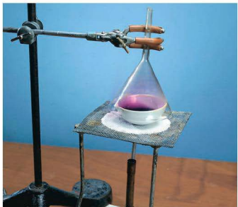
Figure 2.25 Apparatus used to separate an iodine/salt mixture. The iodine sublims on heating.
