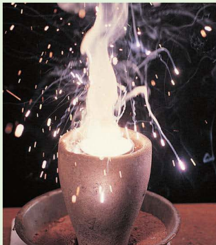
Figure 10.7 The Themit reaction in a laboratory. The same reaction is used to weld damaged railway lines.
