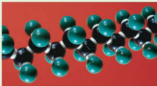
b Model of part of the PTFE polymer chain.
