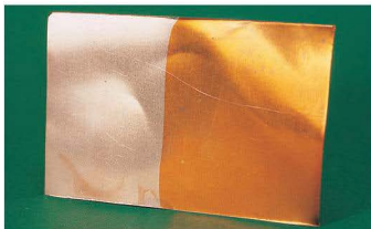
Figure 8.14 Citric acid has been used on the right-hand side of this piece of copper metal to remove the oxide coating on its surface, giving it a shinier appearance.
