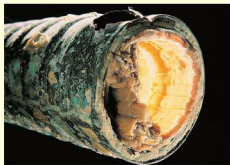
b The thick deposits of limescale can be seen in this hot water pipe. Figure 11.33
