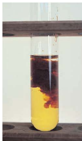
a Iron(III) hydroxide is precipitated. Figure 10.9
