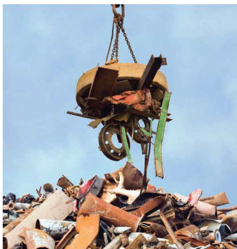
Figure 2.24 Magnetic separation of iron-containing materials.
