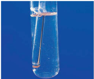
c If the \text{CO}_2 is bubbled for longer the white precipitate dissolves. Figure 13.10 Testing for carbon dioxide.
