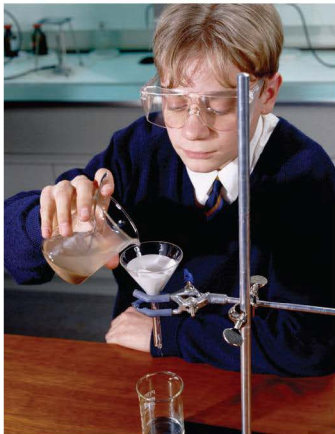
Figure 2.13 It is important when filtering not to overfill the filter paper.
