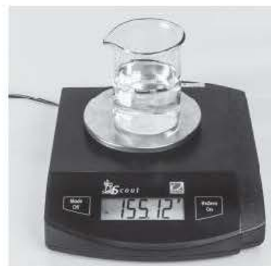
Figure 3 A digital top-pan balance
