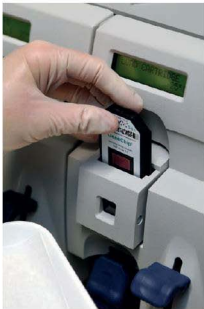
Figure 19.10 Microarray analysis machine with microarray being inserted
