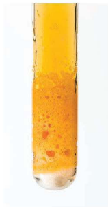
Figure 11.2 Bromine or iodine are the principal products when concentrated sulfuric acid is added to a solid bromide or iodide.
