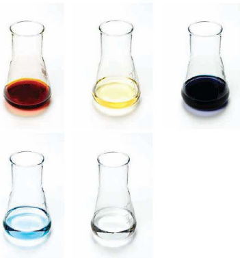
Figure 7.5 The end-point of an iodine titration is made much sharper using starch. A few drops of starch solution are added when the solution is pale yellow; the end-point occurs when the intense blue colour just disappears.
