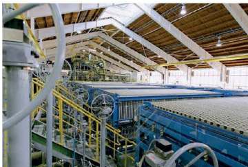
Figure 7.7 Modern plants use a membrane rather than a diaphragm in the cell. This yields very pure sodium hydroxide.
