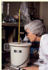
Figure 5.6 Bomb calorimeters are used to measure the energy content not only of fuels but also of foods.
