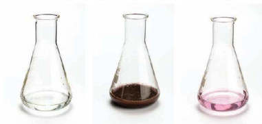
Figure 7.4 To avoid the solution turning brown, warm the solution or use plenty of acid.
