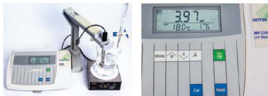
Figure 22.1 In this experimental set-up to record titration curves, the reaction mixture is stirred magnetically and the change in pH is recorded on the meter.
