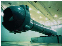
Figure 7.10 Centrifuge testing the effect of acceleration on the human body
