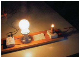
Figure 19.4 A 240 V, 100 W mains lamp is much brighter than a 12 V, 5 W car light, but both have the same current. (Do not try this experiment yourself as it involves a large voltage.)
