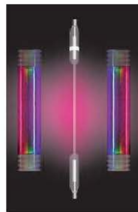
Figure 17.9 Spectra from hydrogen gas discharge tube seen through a diffraction grating.
