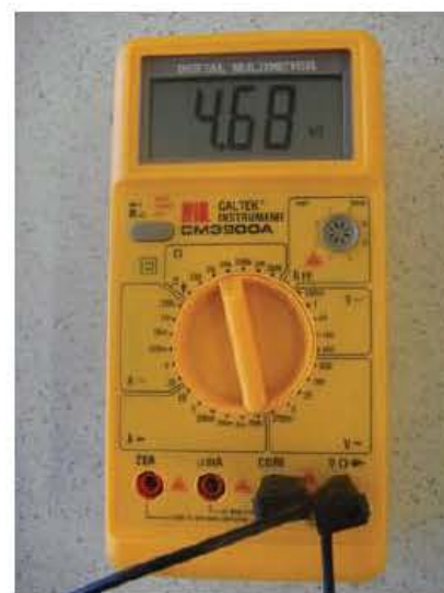
Figure 11.14 Digital multimeter measuring the resistance of a 4.7 \text{ k}\Omega resistor. The meter is set on the 20 \text{ k}\Omega range and so the resistance recorded is 4.68 \text{ k}\Omega .
