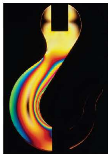
Figure 15.26 Interference stress patterns.
