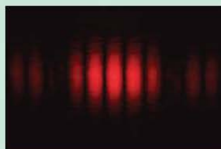
Figure 17.1 Interference fringes from a school laboratory Young's slits experiment using a laser.
