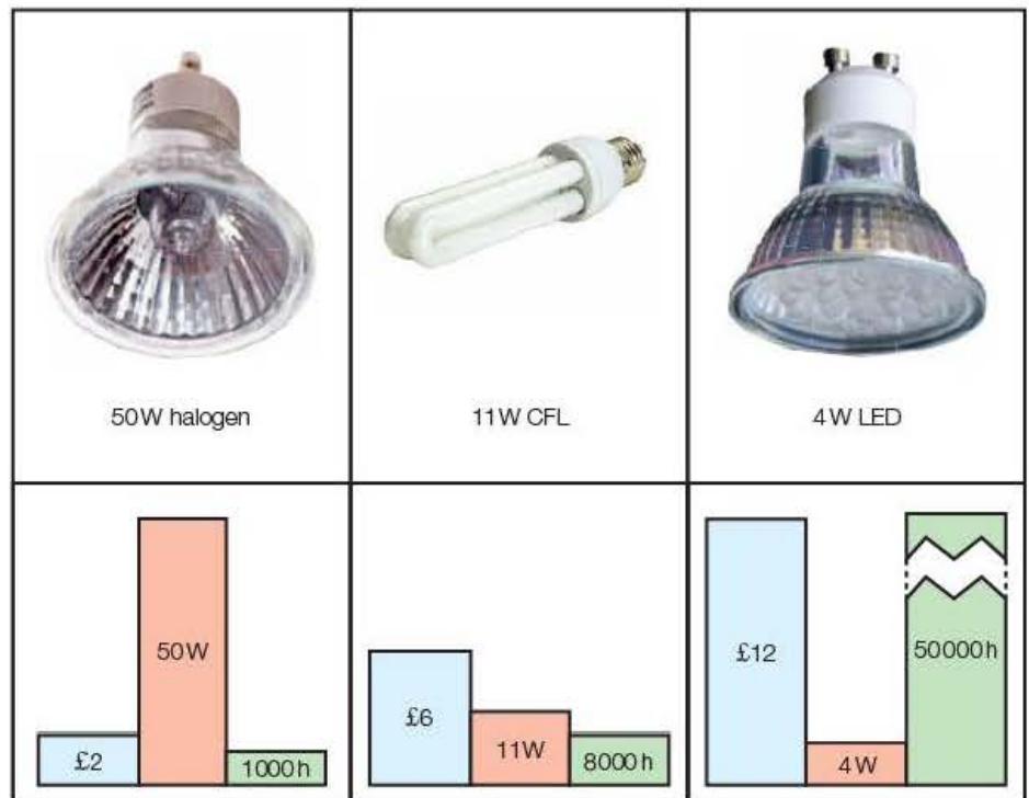
Figure 8.7 Comparison of different types of light bulb.
