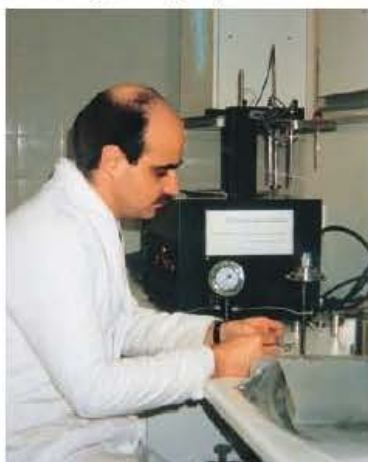
Figure 7.3 Scientists use bomb calorimeters like the one in this photo to measure the energy produced by different fuels and foods.
