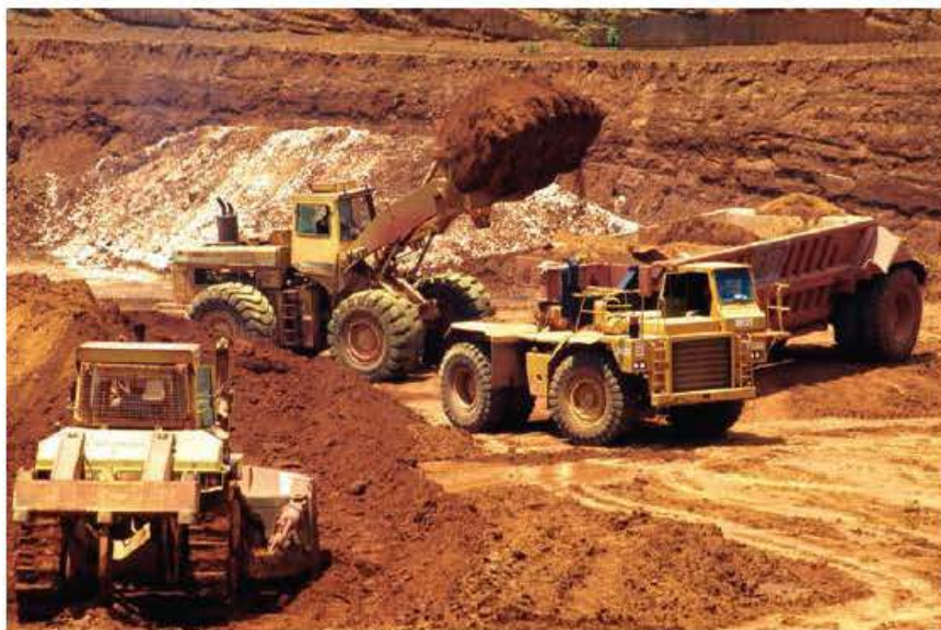
Figure 1.4 Mining bauxite, impure aluminium oxide. Aluminium is extracted from the purified oxide using electrolysis.
