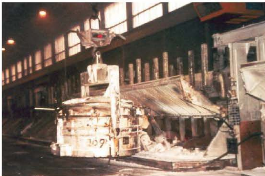
Figure 16.4 Aluminium is manufactured by electrolysis from aluminium oxide. At this factory, molten aluminium is removed from the electrolysis tanks using the suspended and moveable vat shown in the photo.
