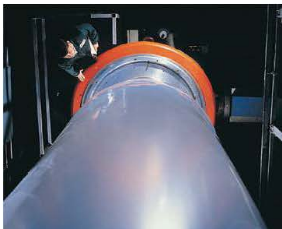
Figure 7.4 Polythene tubing emerging from an extrusion machine. The plastic is extruded from the container in which it is formed by hot pressurised air.
