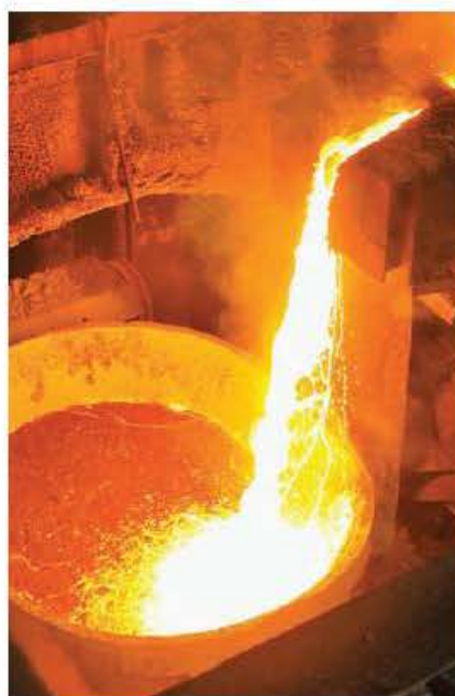
Figure 2.3 Molten iron being poured into a steel-making furnace.
