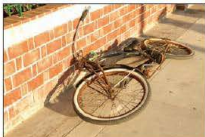
Figure 12.1 Steel parts on a bicycle rust more quickly when the bike is left out in the rain than when it is kept in a shed.
