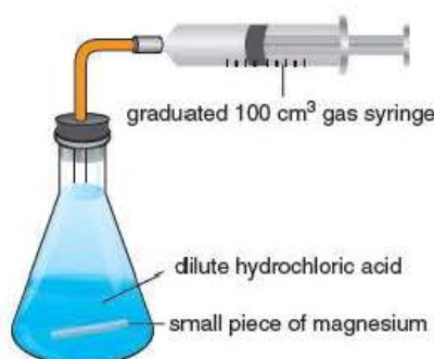
Figure 13.3 Measuring the volume of hydrogen produced when magnesium reacts with dilute hydrochloric acid.
