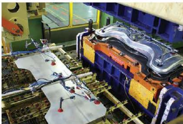
Figure 23.1 This metal press is cold-pressing parts for the body work of a motor car. Why does the metal bend into shape rather than shatter?
