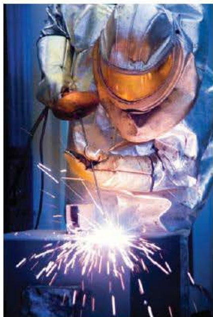
Figure 10.4 Oxy-acetylene flames being used to cut through a large sheet of steel. In oxy-acetylene torches, acetylene burns very rapidly in pure oxygen.
