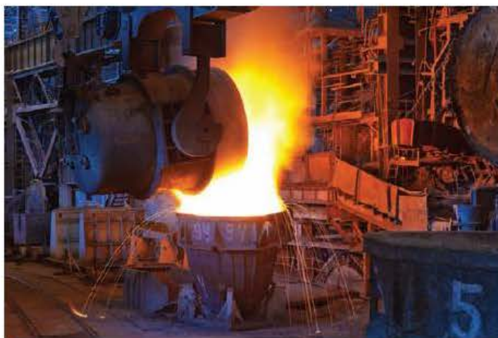
Figure 9.1 Using oxygen to remove impurities from molten iron to make steel.
