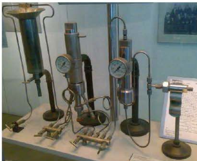
Figure 9.3 The original apparatus used by Fritz Haber to make ammonia.
