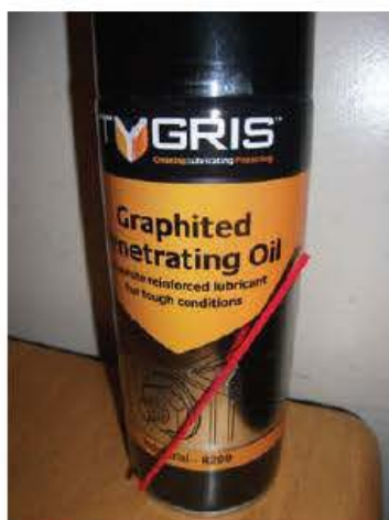
Figure 22.4 A can of lubricating oil containing graphite. Graphite has a layered structure. The layers slip and slide over one another very easily. This makes graphite an excellent material to improve the lubricating action of oils.
