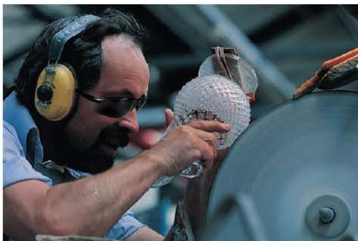
Figure 22.1 Diamonds that are not good enough for jewellery are used in glass cutters and in diamond-studded saws. This photo shows an engraver using a diamond-studded wheel to make patterns in a glass vase.
