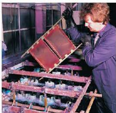
Figure 18.3 Copper-plated sheets being removed from an electroplating bath.
