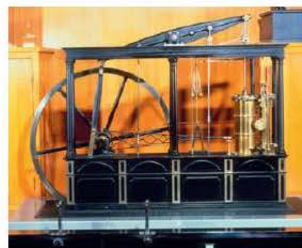
Figure 12.12 ▲ James Watt's steam engine, 1785
