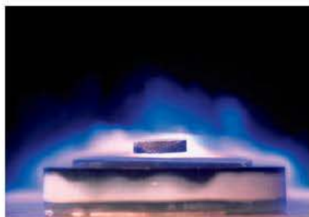
Figure 11.7 ▲ A magnet suspended above a superconducting coil
