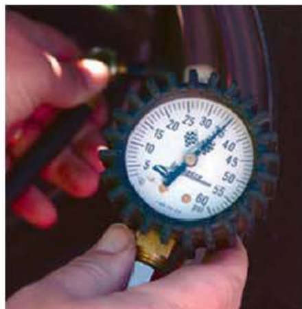
Figure 12.8 ▲ Using a tyre pressure gauge
