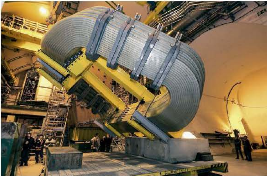
Figure 11.8 ▲ Superconducting electromagnet for the Large Hadron Collider
