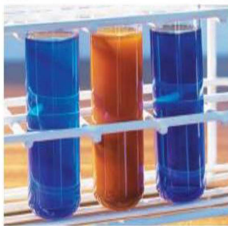
Distinguishing between an aldehyde and a ketone: left, Fehling's solution; centre, Fehling's solution that has been reduced by an aldehyde; right, ketones do not react with Fehling's solution
