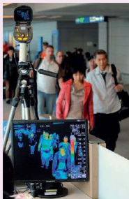
■ Figure 8.53 Thermal scanner at Incheon airport, South Korea
