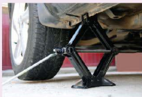
■ Figure 2.111 Changing a car tyre using a simple machine (car jack)
