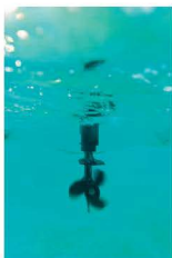
■ Figure 2.135 The propeller at the back of a boat exerts a force on the water and the water pushes back on the propeller
