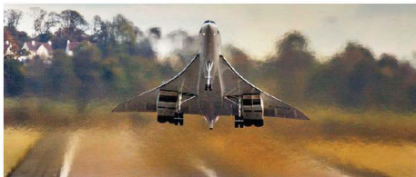
■ Figure 4.65 Diffuse refraction of light by hot gases
