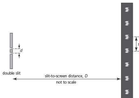
Figure 4.87 Geometry of the double-slit experiment
