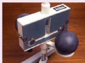
■ Figure 6.22 A modern version Cavendish's apparatus
