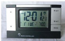
■ Figure 4.51 A seven-segment liquid-crystal display
