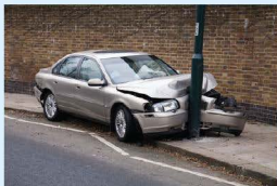
■ Figure 2.119 The front of the car is deformed but the passenger compartment is intact
