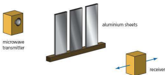
■ Figure 4.84 Interference of microwaves
