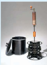
■ Figure 3.18 Joule's apparatus for turning mechanical energy into internal energy.
