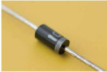
■ Figure 11.43 A typical semi-conductor diode (conventional current flows out of the marked end)
