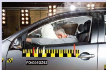
■ Figure 2.118 An air bag greatly reduces the forces in an accident
