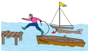
■ Figure 2.92 The force pushing the man forward is equal to the force pushing the boat backwards
