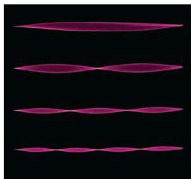
■ Figure 4.93 Standing waves on a stretched string
