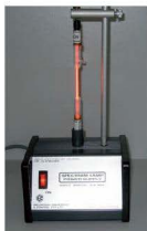
■ Figure 7.1 A discharge tube containing atoms of neon
