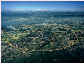
Figure 5.90 The Large Hadron Collider at CERN is underground and has a radius of about 4 km
