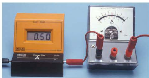
■ Figure 1.2 Digital and analogue ammeters measuring the same electric current
