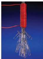
■ Figure 5.73 Testing an electromagnet in a laboratory
