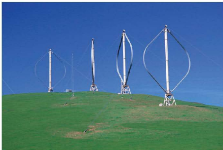
■ Figure 8.29 Wind generators with a vertical axis
