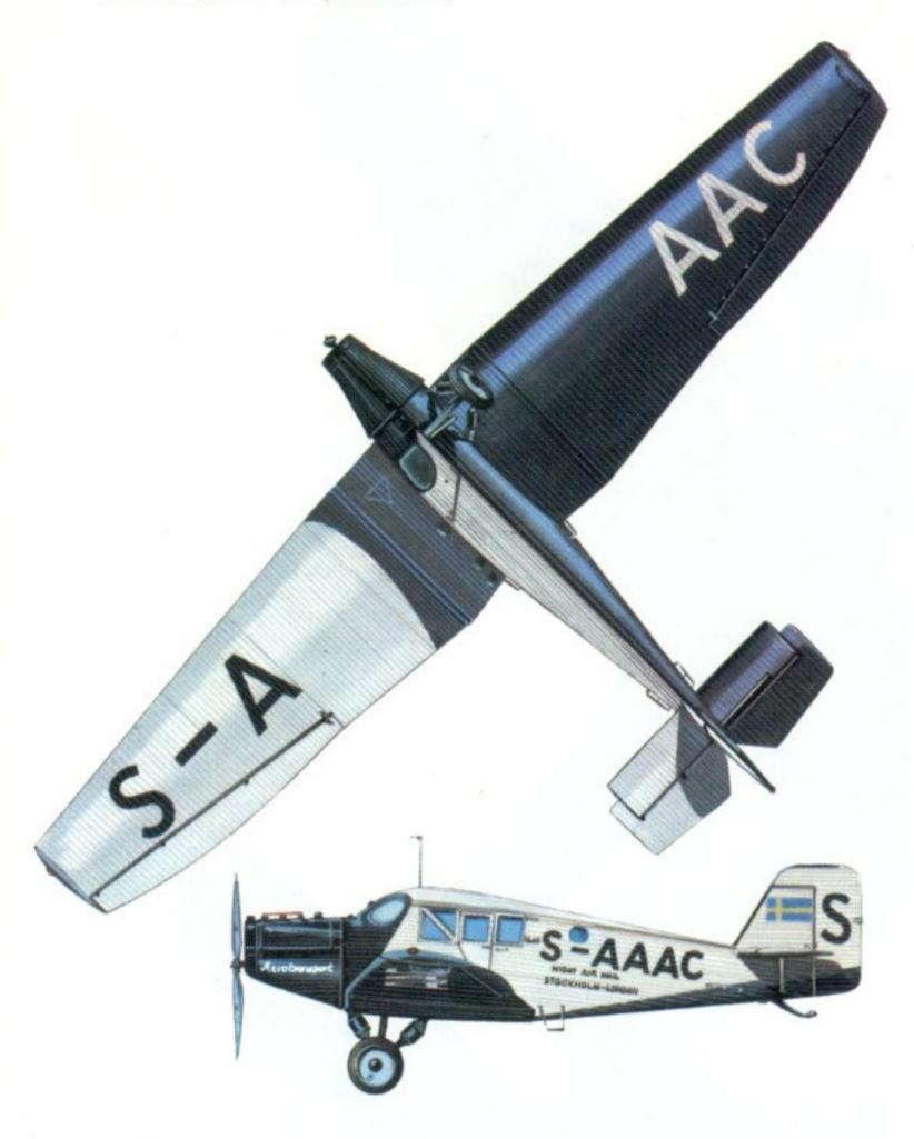
Junkers F 13 of AB Aerotransport, 1928. Engine: One 310 h.p. Junkers L5 six-cylinder in-line. Span: 56 ft. 3½ in. (17.15 m.). Length: 31 ft. 6 in. (9.60 m.). Wing area: 430.6 sq. ft. (40.00 sq. m.). Take-off weight: 4,244 lb. (1,925 kg.). Cruising speed: 99 m.p.h. (160 km/hr.) at 6,560 ft. (2,000 m.). Service ceiling: 8,200 ft. (2,500 m.). Range: 528 miles (850 km.).
