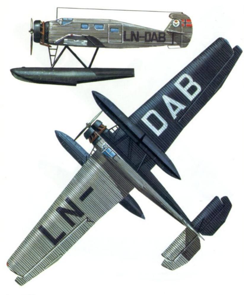
Swedish-built Junkers W 34 Ternen of Det Norske Luftruter, ca 1931. Engine: One 600 h.p. BMW Hornet C nine-cylinder radial. Span: 60 ft. 7½ in. (18.48 m.). Length: 36 ft. 6¼ in. (11.13 m.). Wing area: 473.6 sq.ft. (44.00 sq.m.). Maximum take-off weight: 7,055 lb. (3,200 kg.). Maximum cruising speed: 134 m.p.h. (215 km/hr.) at 3,280 ft. (1,000 m.). Service ceiling: 20,340 ft. (6,200 m.).
