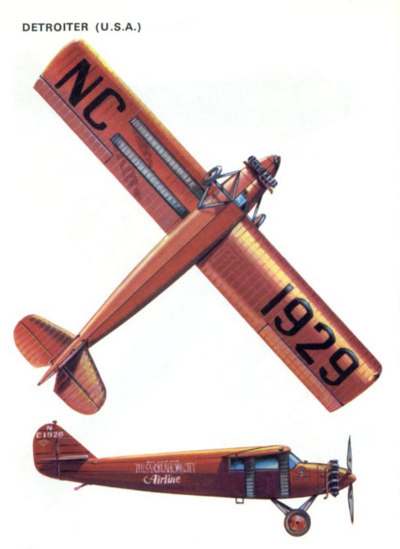
Stinson Model SM-1 Detroiter of Braniff Airways, 1928. Engine: One 220 h.p. Wright Whirlwind J5C nine-cylinder radial. Span: 45 ft. 10 in. (13.97 m.). Length: 32 ft. 10 in. (10.01 m.). Wing area: 292.0 sq.ft. (27.13 sq.m.). Take-off weight: 3,485 lb. (1,580 kg.). Cruising speed: 105 m.p.h. (169 km/hr.). Service ceiling: 14,000 ft. (4,267 m.). Range: 700 miles (1,125 km.).
