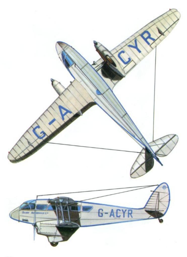
De Havilland D.H.89A Dragon Rapide of Olley Air Service Ltd., 1935. Engines: Two 200 h.p. de Havilland Gipsy Six I six-cylinder in-lines. Span: 48 ft 0 in. (14.63 m.). Length: 34 ft. 6 in. (10.52 m.). Wing area: 336.0 sq.ft. (31.22 sq.m.). Take-off weight: 5,500 lb. (2,495 kg.). Cruising speed: 133 m.p.h. (214 km/hr.). Service ceiling: 16,700 ft. (5,090 m.). Range: 578 miles (930 km.).
