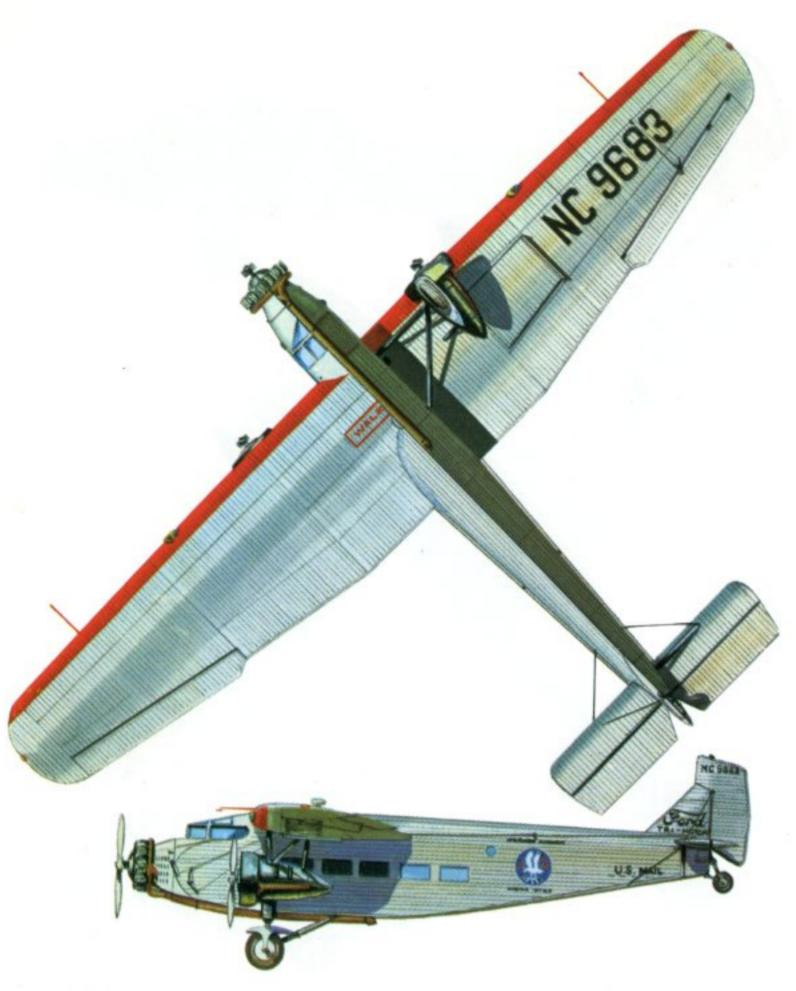
Ford Model 5-AT-B of American Airways, 1931. Engines: Three 420 h.p. Pratt & Whitney Wasp C-1 or SC-1 nine-cylinder radials. Span: 77 ft. 10 in. (23.72 m.). Length: 49 ft. 10 in. (15.19 m.). Wing area: 835.0 sq.ft. (77.57 sq.m.). Typical take-off weight: 13,000 lb. (5,897 kg.). Typical cruising speed: 122 m.p.h. (196 km/hr.) Service ceiling: 18,500 ft. (5,639 m.). Typical range: 550 miles (885 km.).
