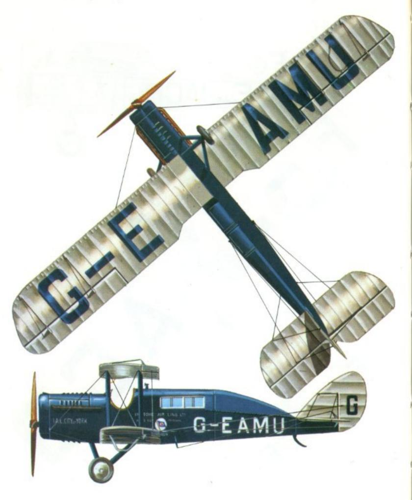
De Havilland D.H.4A City of York of Instone Air Line Ltd, ca late 1922/early 1923. Engine: One 350 h.p. Rolls-Royce Eagle VIII twelve-cylinder Vee type. Span: 42 ft. 4% in. (12.92 m.). Length: 30 ft. 6 in. (9.30 m.). Wing area: 434.0 sq.ft. (40.32 sq.m.). Take-off weight: 3,720 lb. (1,687 kg.). Maximum speed: 121 m.p.h. (195 km/hr.). Service ceiling: approx 20,000 ft. (6,100 m.). Range: 250 miles (402 km.).
