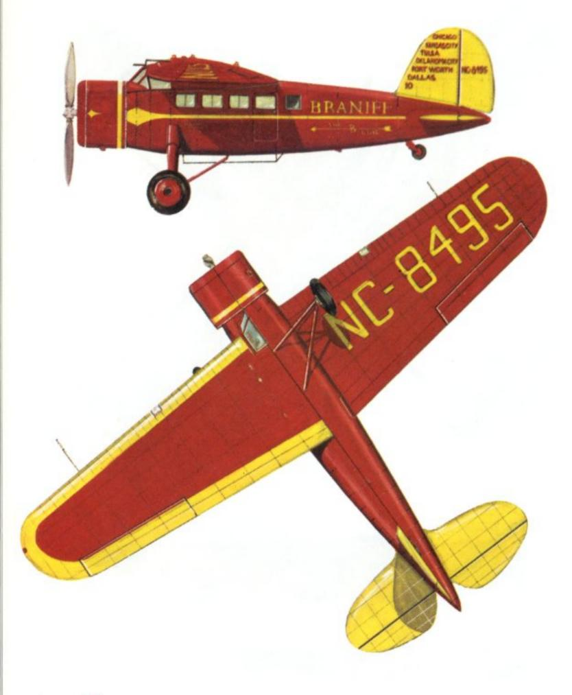
Lockheed Vega Model DL-1 of Braniff Airways, ca 1934-35. Engine: One 450 h.p. Pratt & Whitney Wasp C1 nine-cylinder radial. Span: 41 ft. 0 in. (12.50 m.). Length: 27 ft. 6 in. (8.38 m.). Wing area: 275.0 sq. ft. (25.55 sq. m.). Take-off weight: 4,270 lb. (1,937 kg.). Cruising speed: 150 m.p.h. (241 km/hr.). Service ceiling: approx 22,000 ft. (6,705 m.). Range: approx 700 miles (1,126 km.)
