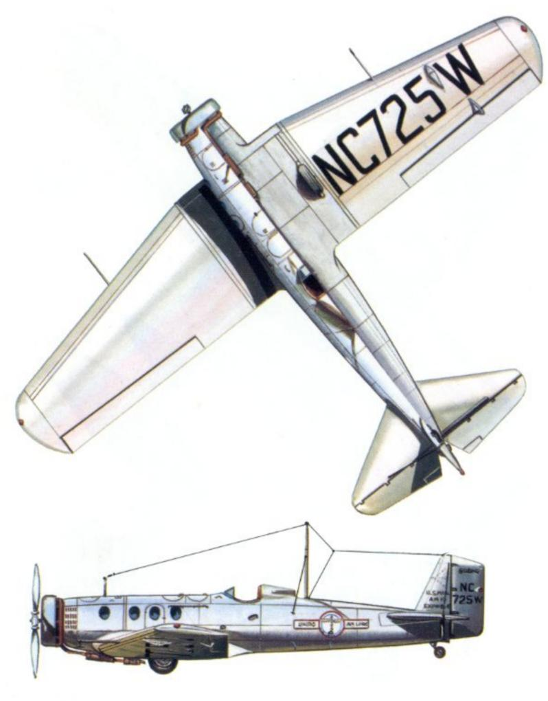
Boeing Model 221A (originally Model 200) Monomail of United Air Lines (Boeing Air Transport Division), ca 1932. Engine: One 575 h.p. Pratt & Whitney Hornet B nine-cylinder radial. Span: 59 ft. 1½ in. (18.02 m.). Length: 44 ft. 1½ in. (13.45 m.). Wing area: 535.0 sq.ft. (49.70 sq.m.). Take-off weight: 8,000 lb. (3,629 kg.). Cruising speed: 137 m.p.h. (220 km/hr.). Service ceiling: 14,700 ft. (4,480 m.). Range: 540 miles (869 km.).
