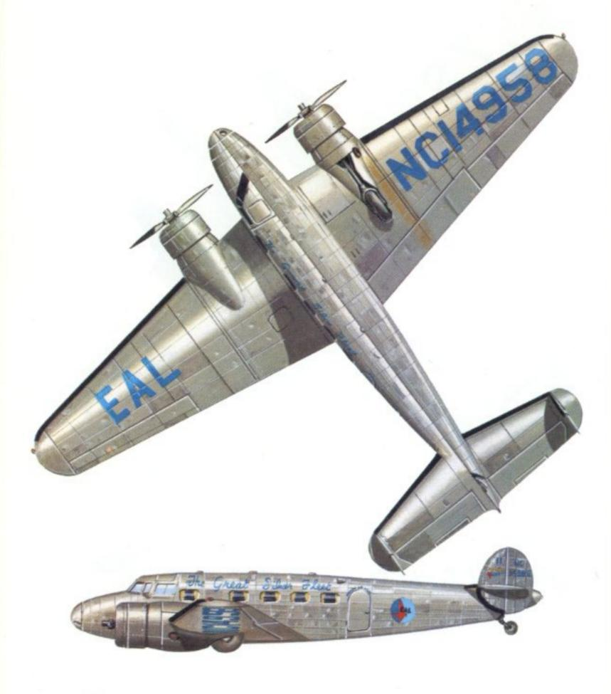
Lockheed Model 10 Electra of Eastern Air Lines, ca 1934-35. Engines: Two 440 h.p. Wright R-975-E3 Whirlwind nine-cylinder radials. Span: 55 ft. 0 in. (16.76 m.). Length: 38 ft. 7 in. (11.76 m.). Wing area: 458.5 sq.ft. (42.60 sq.m.). Take-off weight: 9,750 lb. (4,423 kg.). Cruising speed: 182 m.p.h. (293 km/hr.) at 5,000 ft. (1,524 m.). Service ceiling: 21,650 ft. (6,600 m.). Range: 810 miles (1,304 km.).
