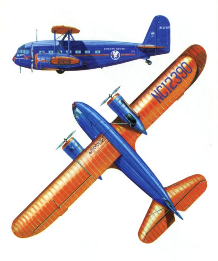
Curtiss Model AT-32-A Condor of American Airways, 1934. Engines: Two 710 h.p. Wright Cyclone SGR-1820-F3 nine-cylinder radials. Span: 82 ft. 0 in. (24.99 m.). Length: 48 ft. 7 in. (14.81 m.). Wing area: 1,208.0 sq.ft. (112.22 sq.m.). Take-off weight: 17.500 lb. (7,938 kg.). Speed: 167 m.p.h. (269 km/hr.) at 8,000 ft. (2,438 m.). Service ceiling: 23,000 ft. (7,010 m.). Maximum range: 716 miles (1,152 km.).
