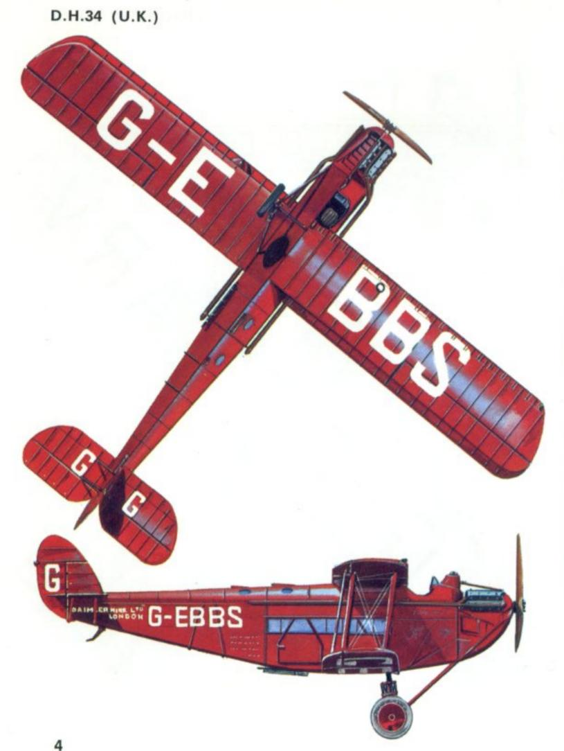
De Havilland D.H.34 of Daimler Hire Ltd, 1922. Engine: One 450 h.p. Napier Lion twelve-cylinder 'broad arrow type. Span: 51 ft. 0 in. (15.54 m.). Length: 39 ft. 0 in. (11.89 m.). Wing area: 590.0 sq.ft. (54.81 sq.m.). Take-off weight: 7,200 lb. (3,266 kg.). Cruising speed: 105 m.p.h. (169 km/hr.). Service ceiling: 14,500 tt. (4,420 m.). Range: 365 miles (587 km.).
