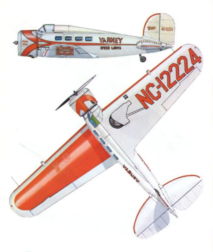
Lockheed Model 9 Orion South Wind of Varney Speed Lanes, 1930. Engine: One 450 h.p. Pratt & Whitney Wasp S1D1 nine-cylinder radial. Span: 42 ft. 9½ in. (13.04 m.). Length: 27 ft. 6 in. (8.38 m.). Wing area: 294.1 sq.ft. (27.32 sq.m.). Take-off weight (mail version): 5,400 lb. (2,449 kg.). Cruising speed: 175 m.p.h. (282 km/hr.) at 11,000 ft. (3,353 m.). Service ceiling: 22,000 ft. (6,706 m.). Range: 750 miles (1,207 km.).
