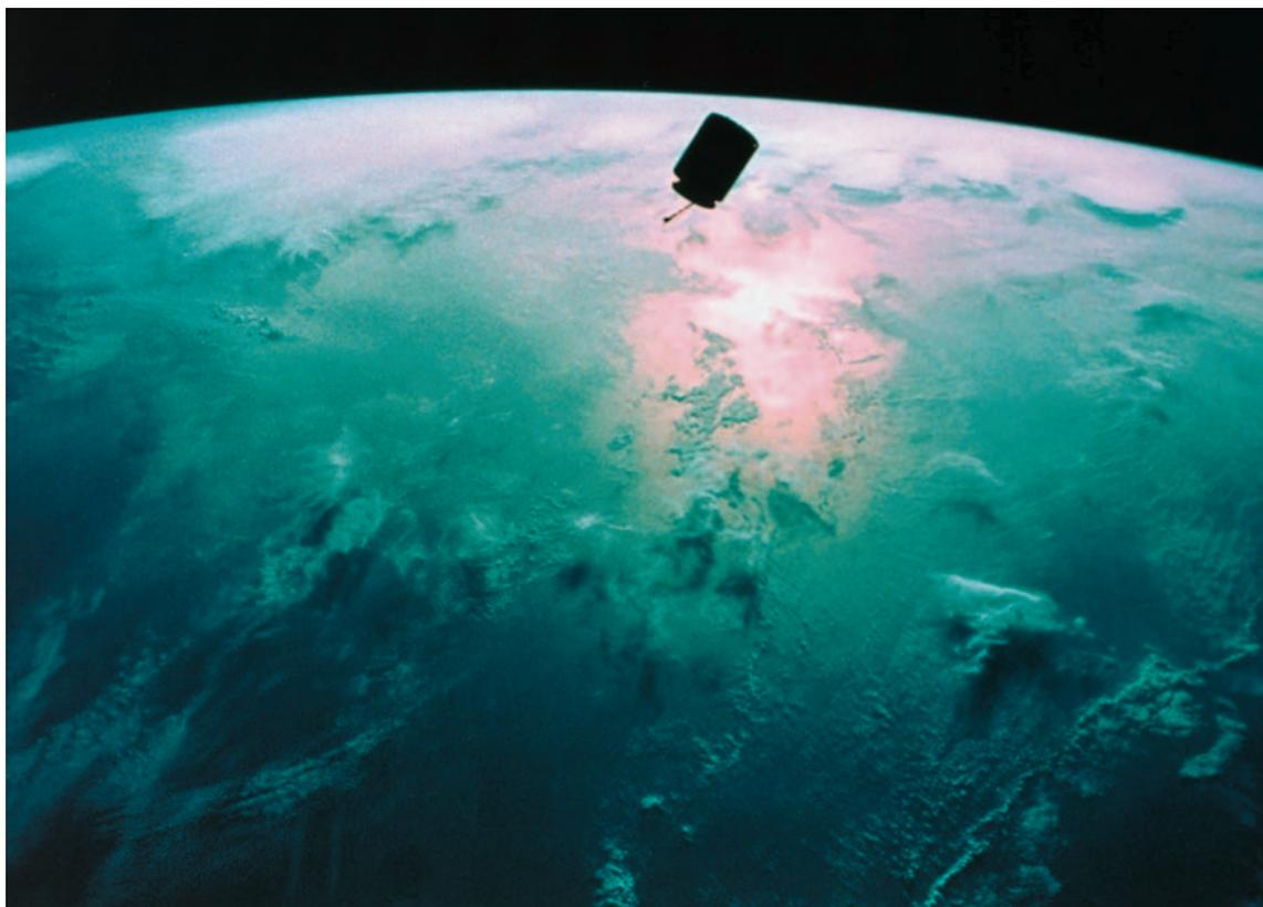
**Intelsat VI floating over the Earth. Within hours of this shot, astronauts grabbed the satellite, attached a perigee stage, and released it back into space.** U.S. National Aeronautics and Space Administration (NASA).
