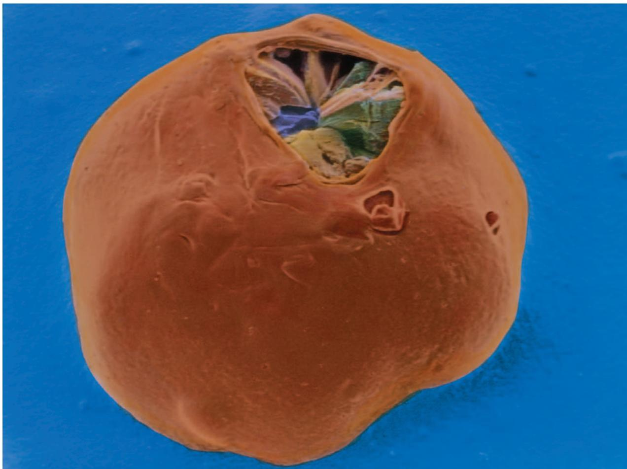
A scanning electron micrograph (SEM) of the surface of a sheet of biodegradable plastic. The spherical object that dominates the image is one of many granules of starch embedded in the surface of the plastic. When the plastic is buried in soil the starch grains take up water and expand. This breaks the material into small fragments, increasing the contact area with the soil bacteria that digest plastic. *National Audubon Society Collection/Photo Researchers, Inc. Reproduced by permission.*
