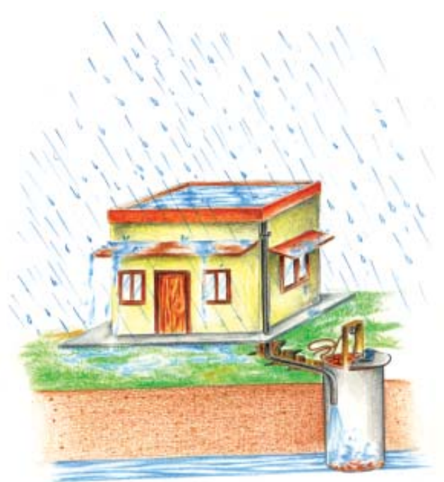
(b) Recharge through Abandoned Dugwell
