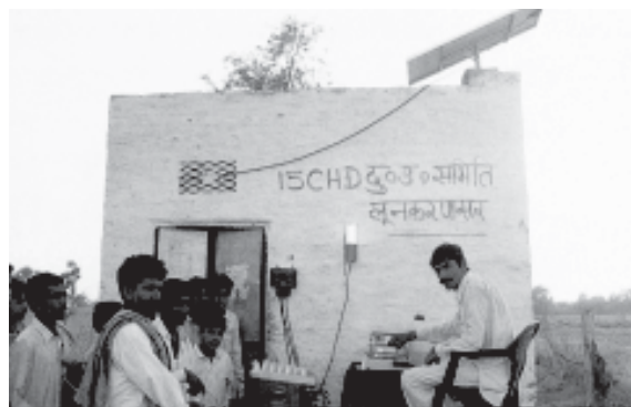
Fig. 5.12: Solar operated electronic milk testing equipment
