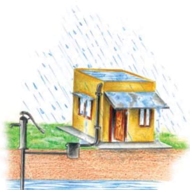
(a) Recharge through Hand Pump
