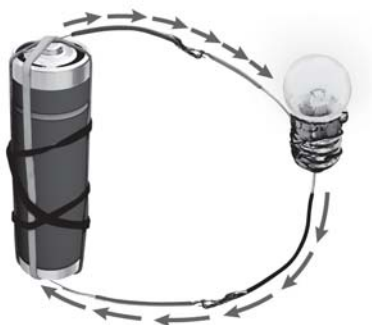
Fig.12.6 Direction of current in an electric circuit
