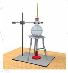
**Fig. 8.1**: Determination of Boiling point of water
