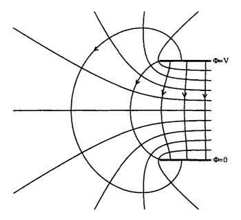
(d) Bonus. Calculate the charge density on the conducting surfaces. Use your result to find the induced charge on the conductor (of finite length), and thus the capacitance of this arrangement. Compare your result to the "infinite" parallel plate capacitor and comment on the influence of "fringing" fields on the calculation of the capacitance.
