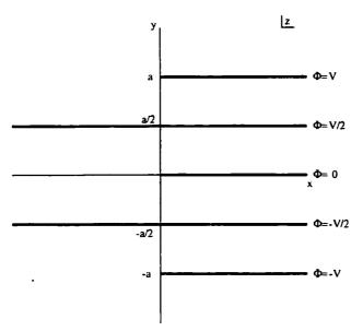
We can think of this either as a periodic array of semi-infinite conducting plates at y = na, held at potentials  $nV_0$ , or as an infinite parallel plate capacitor, with plates located at  $y = \pm a/2$ , with a semi-infinite conductor stuck halfway in between. We'll stick with the former interpretation, and confine attention to values of the potential between 0 and  $V_0$  (essentially ignoring the periodicity).
