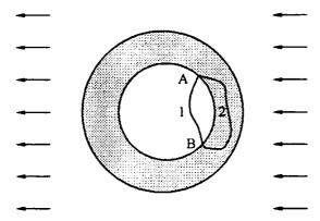
(c) The electric field at the exterior surface of a charged conductor is normal to the surface and has a magnitude  $\sigma(\mathbf{x})/\epsilon_0$ , where  $\sigma(\mathbf{x})$  is the local surface charge density.
