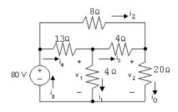
$$\begin{split} v_2 &= 2(20) = 40 \text{ V} \\ v_{8\Omega} &= 80 - 40 = 40 \text{ V} \\ i_2 &= 40 \text{ V}/8 \,\Omega = 5 \text{ A} \\ i_3 &= i_o - i_2 = 2 - 5 = -3 \text{ A} \\ v_{4\Omega} &= (-3)(4) = -12 \text{ V} \\ v_1 &= 4i_3 + v_2 = -12 + 40 = 28 \text{ V} \\ i_1 &= 28 \text{ V}/4 \,\Omega = 7 \text{ A} \end{split}$$
