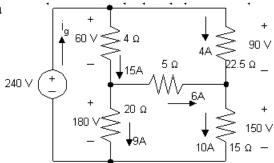
Calculate the power dissipated by the resistors using the equation  $p_R = Ri_R^2$ :
