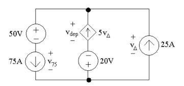
Write the two KCL equations, summing the currents leaving the node:
