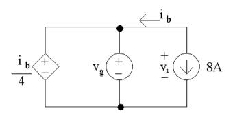
[a] To find  $v_g$  write a KVL equation clockwise around the left loop, starting below the dependent source:
