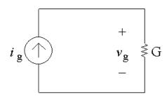
[a] Note from the circuit that the current throught the conductance G is  $i_g$ , flowing from top to bottom (from KCL), and the voltage drop across the current source is  $v_g$ , positive at the top (from KVL). From a version of Ohm's law,
