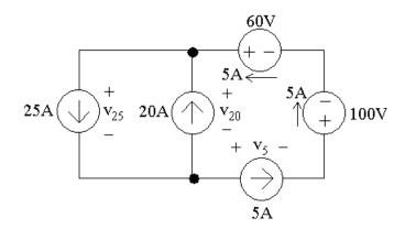
Write the two KCL equations, summing the currents leaving the node:
