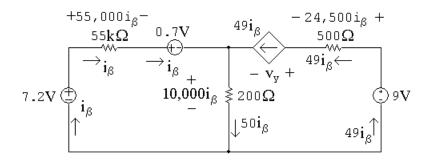
[a] To find  $i_{\beta}$ , write a KVL equation around the left-hand loop, summing voltages in a clockwise direction starting below the 7.2V source:
