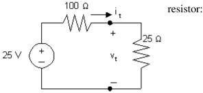
To find the power delivered to the  $25\,\Omega$  resistor we must calculate the current through the  $25\,\Omega$  resistor. Do this by first using KCL to recognize that the current in each of the components is  $i_t$ , flowing in a clockwise direction. Write a KVL equation in the clockwise direction, starting below the voltage source, and using Ohm's law to express the voltage drop across the resistors in the direction of the current  $i_t$  flowing through the resistors:
