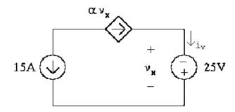
[a] Note from the circuit that  $v_x = -25$  V. To find  $\alpha$  write a KCL equation at the top left node, summing the currents leaving:
