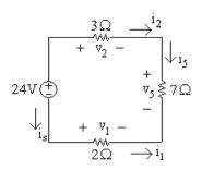
Write a KVL equation clockwise around the circuit, starting below the voltage source:
