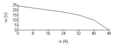
**[b]** Since the plot is linear for  $0 \le i_s \le 24$  A and since  $R = \Delta v/\Delta i$ , we can calculate R from the plotted values as follows:
