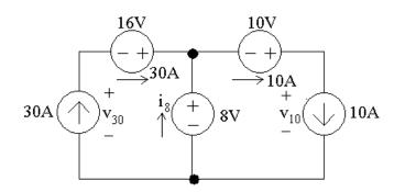
Write the two KCL equations, summing the currents leaving the node:
