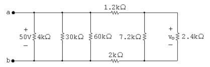
The voltage drop across the  $4~k\Omega$  resistor is the same as the voltage drop across the series combination of the  $1.2~k\Omega$ , the  $(7.2~k\|2.4~k)\Omega$  combined resistor, and the  $2~k\Omega$  resistor. Note that
