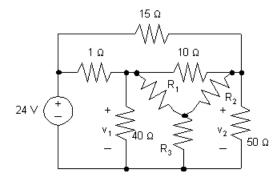
Now use Eqs. 3.44 - 3.46 to calculate the values of the  $\Delta$ -connected resistors:
