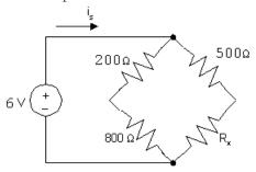
The condition for a balanced bridge is that the product of the opposite resistors must be equal:
