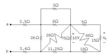
The equivalent resistance of the  $5\,\Omega$ ,  $15\,\Omega$ , and  $60\,\Omega$  resistors is
