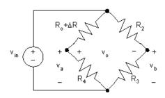
$$v_{\rm a} = \frac{v_{\rm in}R_4}{R_o + R_4 + \Delta R}$$
