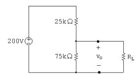
[a] We can use voltage division to calculate the voltage  $v_o$  across the 75 k $\Omega$  resistor:
