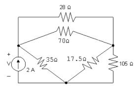
From this circuit we see that the  $70\,\Omega$  resistor is parallel to the  $28\,\Omega$  resistor:
