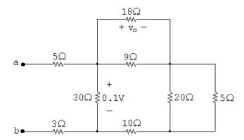
First, note the following:  $18\|9=6\,\Omega;\,20\|5=4\,\Omega;$  and the voltage drop across the  $18\,\Omega$  resistor is the same as the voltage drop across the parallel combination of the  $18\,\Omega$  and  $9\,\Omega$  resistors. Using voltage division,
