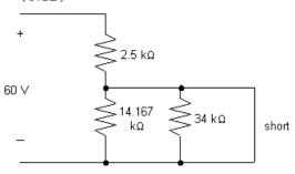
Maximum dissipation in  $R_2$  occurs at no load, therefore,
