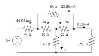
$$i_{80\Omega} = 44.04 \text{ m} - 23.65 \text{ m} = 20.39 \text{ mA}$$
