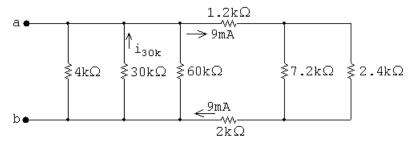
The 9 mA current in the  $1.2~k\Omega$  resistor is also the current in the  $2~k\Omega$  resistor. It then divides among the  $4~k\Omega$ ,  $30~k\Omega$ , and  $60~k\Omega$  resistors.
