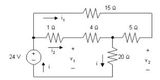
The equivalent resistance seen by the 24 V source can be calculated by making series and parallel combinations of the resistors to the right of the 24 V source:
