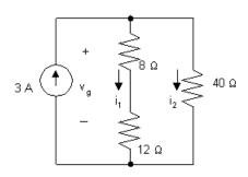
$$i_1 = \frac{(3)(40)}{(60)} = 2 \text{ A}; \qquad v_x = 8i_1 = 16 \text{ V}$$
