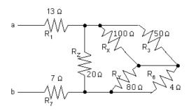
Make series and parallel combinations of the resistors to find the equivalent resistance  $R_{\rm ab}$ :
