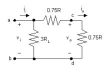
$$i_o = \frac{i_i(3R_{\rm L})}{4.5R_{\rm L}} = \frac{1}{1.5}i_i = \frac{1}{1.5}\frac{v_i}{R_{\rm L}}, \qquad v_o = 0.75R_{\rm L}i_o = \frac{1}{2}v_i,$$
