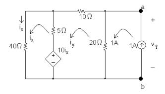
The mesh current equations for the two meshes on the left:
