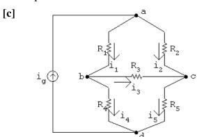
Sum the currents at any three of the four essential nodes a, b, c, and d. Using nodes a, b, and c we get
