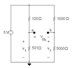
Use voltage division to calculate  $v_1$  and  $v_2$ :
