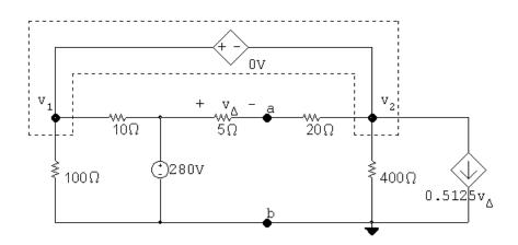
$$\begin{split} \frac{v_1}{100} + \frac{v_1 - 280}{10} + \frac{v_1 - 280}{25} + \frac{v_1}{400} + 0.5125v_{\Delta} &= 0 \\ v_{\Delta} = \frac{(280 - v_1)}{25} 5 = 56 - 0.2v_1 \\ v_1 &= 210 \text{ V}; \qquad v_{\Delta} = 14 \text{ V} \\ V_{\text{Th}} &= 280 - v_{\Delta} = 280 - 14 = 266 \text{ V} \end{split}$$
