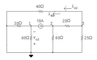
$$\frac{v_1}{30} + \frac{v_1}{60} + 18 = 0$$
