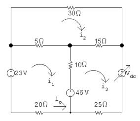
Write the mesh current equations. Note that if  $i_0 = 0$ , then  $i_1 = 0$ :
