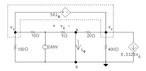
$$\frac{v_1}{100} + \frac{v_1 - 280}{10} + \frac{v_2}{20} + \frac{v_2}{400} + 0.5125(280) = 0$$
