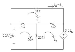
Since the bottom left mesh current value is known, we need only two mesh current equations:
