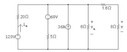
Transform the  $120~\rm V$  source in series with the  $20~\Omega$  resistor into a  $6~\rm A$  source in parallel with the  $20~\Omega$  resistor. Also transform the  $-60~\rm V$  source in series with the  $5~\Omega$  resistor into a  $-12~\rm A$  source in parallel with the  $5~\Omega$  resistor. The result is the following circuit:
