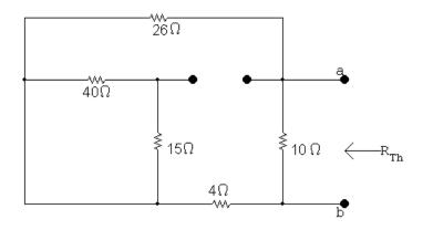
$$R_{\rm Th} = 10 \| (26 + 4) = 7.5 \,\Omega \, (\text{CHECKS})$$
