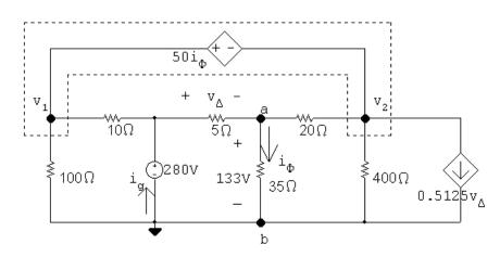
$$\frac{v_1}{100} + \frac{v_1 - 280}{10} + \frac{v_2 - 133}{20} + \frac{v_2}{400} + 0.5125(280 - 133) = 0$$
