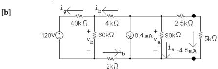
$$\begin{array}{lll} v_{\rm a} & = & (7500)(-0.0045) = -33.75 \ {\rm V} \\ i_{\rm a} & = & \frac{v_{\rm a}}{90,000} = \frac{-33.75}{90,000} = -0.375 \ {\rm mA} \\ i_{\rm b} & = & -8.4 \times 10^{-3} + 0.375 \times 10^{-3} + 4.5 \times 10^{-3} = -3.525 \ {\rm mA} \\ v_{\rm b} & = & (6000)(3.525 \times 10^{-3}) - 33.75 = -12.6 \ {\rm V} \\ i_g & = & \frac{-12.6 - 120}{40,000} = -3.315 \ {\rm mA} \\ p_{120{\rm V}} & = & (120)(-3.315 \times 10^{-3}) = -397.8 \ {\rm mW} \end{array}$$
