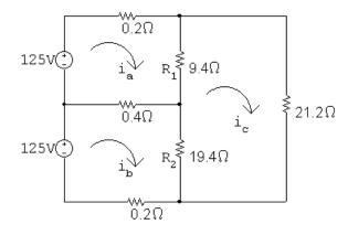
$$125 = (R_1 + 0.6)i_a - 0.4i_b - R_1i_c$$
