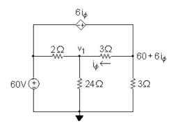
The node voltage equation at  $v_1$  is
