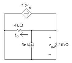
$$\frac{v_{o2}}{4000} + \frac{v_{o2}}{20,000} + 0.005 - 2.2\left(\frac{v_{o2}}{4000}\right) = 0$$
