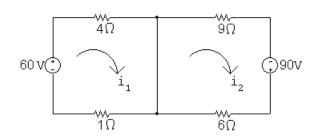
Now there is no longer a supermesh. The two simple mesh current equations are:
