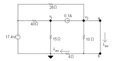
Write a node voltage equation at  $v_2$ :
