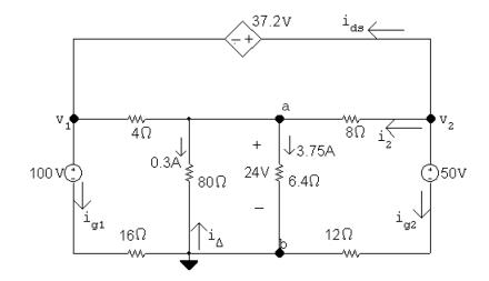
Using the node voltage method to find  $v_1$  and  $v_2$  yields
