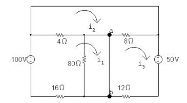
Note with the short circuit from a to b that  $i_{\Delta}$  is zero, hence  $124i_{\Delta}$  is also zero. The mesh currents are:
