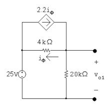
$$\frac{v_{o1} - 25}{4000} + \frac{v_{o1}}{20,000} - 2.2\left(\frac{v_{o1} - 25}{4000}\right) = 0$$
