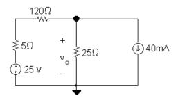
Note that we have chosen the lower node as the reference node, and that the voltage at the upper node with respect to the reference node is  $v_o$ . Write a KCL equation (node voltage equation) by summing the currents leaving the upper node:
