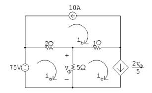
There are current sources on the perimeters of both the  $i_{\rm b}$  mesh and the  $i_{\rm c}$  mesh, so we know that
