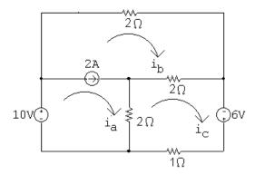
The 2 A current source is shared by the meshes  $i_{\rm a}$  and  $i_{\rm b}$ . Thus we combine these meshes to form a supermesh and write the following equation:
