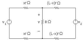
$$\frac{v - v_1}{2xr} + \frac{v}{R} + \frac{v - v_2}{2r(L - x)} = 0$$
