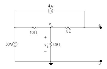
Write and solve the node voltage equation at  $v_1$ :
