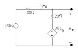
$$i_{\Delta} = \frac{160 - 30i_{\Delta}}{50}; \qquad i_{\Delta} = 2 \text{ A}$$
