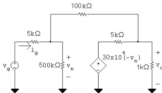
Write two node voltage equations, one at the left node, the other at the right node:
