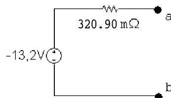
[b] The output resistance of the inverting amplifier is the same as the Thévenin resistance, i.e.,
