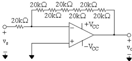
Alternately, Use a single  $20 \text{ k}\Omega$  resistor as the feedback resistor and use six  $20 \text{ k}\Omega$  resistors in parallel as the input resistor to give a total of  $3.33 \text{ k}\Omega$ .
