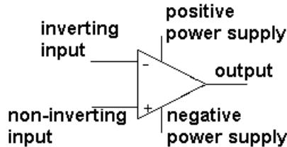
[b] The input resistance of an ideal op amp is infinite, which constrains the value of the input currents to 0. Thus,  $i_n = 0 \text{ A}$ .
