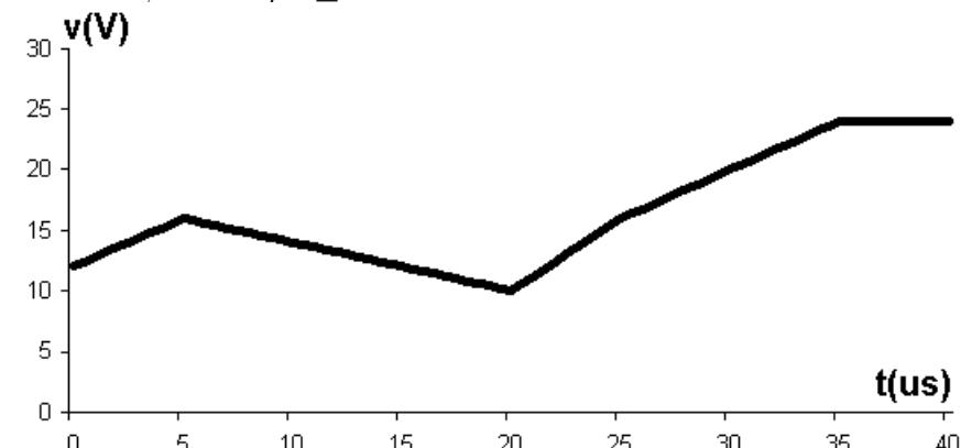
P 6.16  $v = -10 \text{ V}, \quad t \leq 0; \quad C = 0.8 \mu\text{F}$
