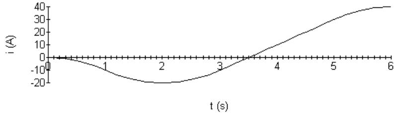
P 6.6 [a]  $v_L = L \frac{di}{dt} = [125 \sin 400t] e^{-200t} \text{ V}$
