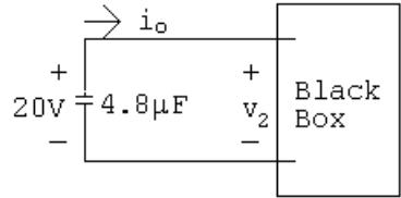
$$\begin{aligned} v_2 &= -\frac{1}{4.8 \times 10^{-6}} \int_0^t 1.92 \times 10^{-3} e^{-20x} dx + 20 \\ &= -400 \frac{e^{-20x}}{-20} \Big|_0^t + 20 \\ &= 20(e^{-20t} - 1) + 20 \\ &= 20e^{-20t} \text{ V}, \quad t \geq 0 \end{aligned}$$
