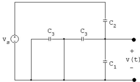
$$C_1 \frac{dv}{dt} + C_3 \frac{dv}{dt} + C_2 \frac{d(v - v_s)}{dt} = 0$$
