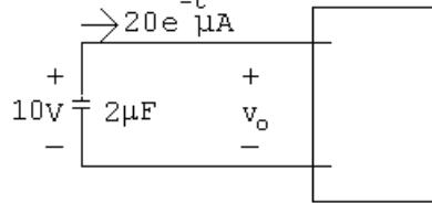
$$\begin{aligned} v_o &= -\frac{1}{2 \times 10^{-6}} \int_0^t 20 \times 10^{-6} e^{-x} dx + 10 \\ &= 10e^{-x} \Big|_0^t + 10 \\ &= 10e^{-t} \text{V}, \quad t \geq 0 \end{aligned}$$
