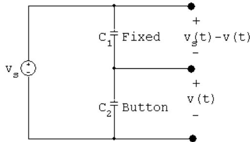
$$C_2 \frac{dv}{dt} = C_1 \frac{d}{dt}(v_s - v)$$
