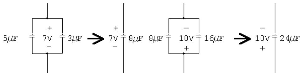
$$\frac{1}{24} + \frac{1}{8} = \frac{4}{24} \quad \therefore C_{\text{eq}} = 6 \mu\text{F}$$
