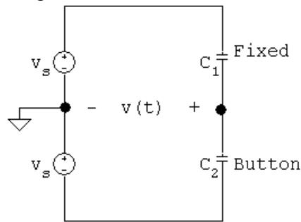
$$C_1 \frac{dv}{dt} (v - v_s) + C_2 \frac{d}{dt} (v + v_s) = 0$$
