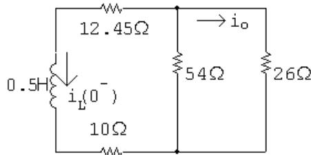
$$i_L(t) = i_L(0^+)e^{-t/\tau} \text{ A}, \quad t \geq 0$$
