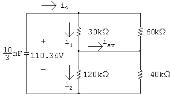
$$R_e = 30\parallel 60 + 120\parallel 40 = 20 + 30 = 50 \text{ k}\Omega$$
