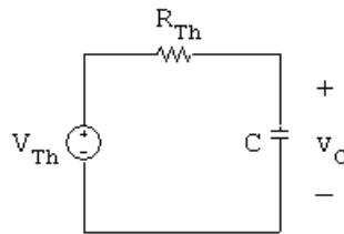
$$R_{\text{Th}} = R \parallel R_L = \frac{RR_L}{R + R_L}; \quad V_{\text{Th}} = \frac{R_L}{R + R_L} V_s$$
