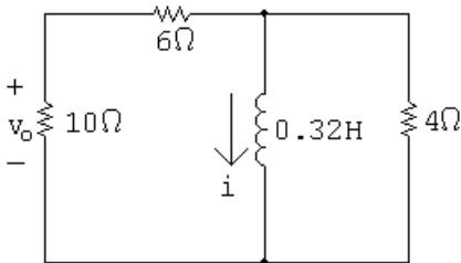
$$R_{\text{eq}} = 4 \parallel (6 + 10) = 3.2 \Omega, \quad \therefore \quad \tau = \frac{L}{R_{\text{eq}}} = \frac{0.32}{3.2} = 0.1 \text{ s}$$
