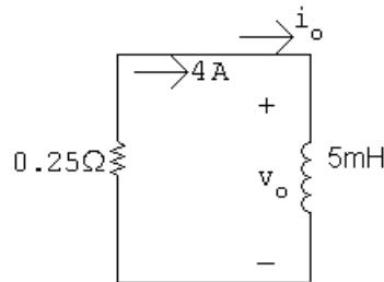
$$i_o = 4e^{-50t} \text{ A}, \quad t \geq 0$$
