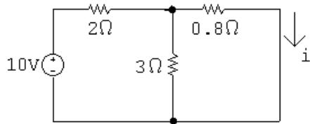
The equivalent resistance seen by the 10 V source is  $2 + (3\parallel 0.8)$ . The current leaving the 10 V source is
