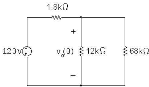
$$R_e = 12 \text{ k} \parallel 68 \text{ k} = 10.2 \text{ k}\Omega$$
