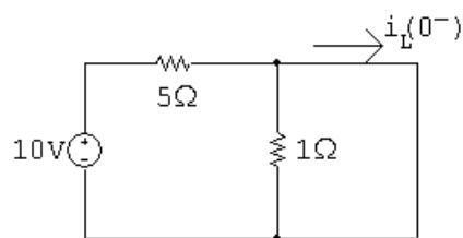
$$i_L(0^-) = 10 \text{ V}/5 \Omega = 2 \text{ A} = i_L(0^+)$$
