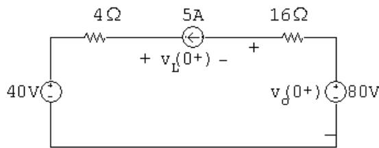
$$v_L(0^+) = 40 + (5 \text{ A})(4 \Omega) = 60 \text{ V}, \quad v_o(0^+) = 80 - (16 \Omega)(5 \text{ A}) = 0 \text{ V}$$
