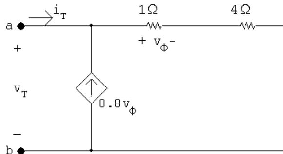
$$v_T = (i_T + 0.8v_\phi)(5) = \left( i_T + 0.8 \frac{v_T}{5} \right) (5)$$
