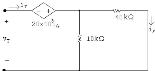
$$v_T = -20 \times 10^3 i_\Delta + 8 \times 10^3 i_T = -20 \times 10^3 (0.2) i_T + 8 \times 10^3 i_T = 4 \times 10^3 i_T$$
