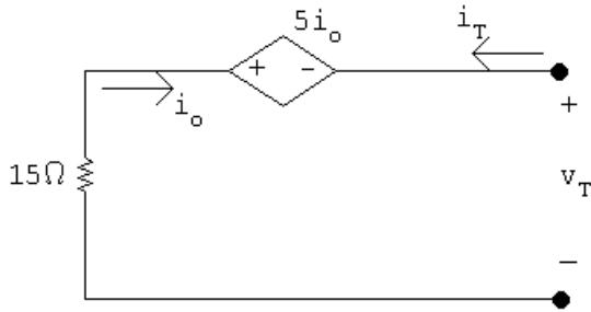
$$v_T = -5i_o - 15i_o = -20i_o = 20i_T \quad \therefore \quad R_{Th} = \frac{v_T}{i_T} = 20\Omega$$
