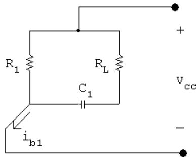
$$i_{b1} = \frac{V_{CC}}{R_1} + \frac{V_{CC}}{R_L} e^{-t/R_L C_1}$$
