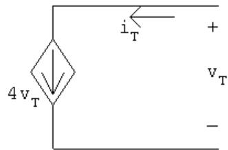
$$i_T = 4v_T; \quad \frac{v_T}{i_T} = R_{\text{Th}} = \frac{1}{4} = 0.25 \Omega$$
