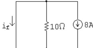
Note that the inductor behaves as a short circuit and all of the current from the 8 A source flows through the short circuit. Thus,
