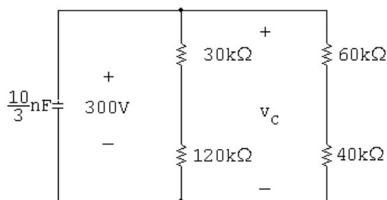
$$R_e = 150 \parallel 100 = 60 \text{ k}\Omega; \quad \tau = \left(\frac{10}{3} \times 10^{-9}\right)(60,000) = 200 \mu\text{s}$$
