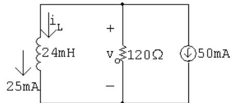
$$i_L(0^-) = i_L(0^+) = 25 \text{ mA}; \quad \tau = \frac{24 \times 10^{-3}}{120} = 0.2 \text{ ms}; \quad \frac{1}{\tau} = 5000$$
