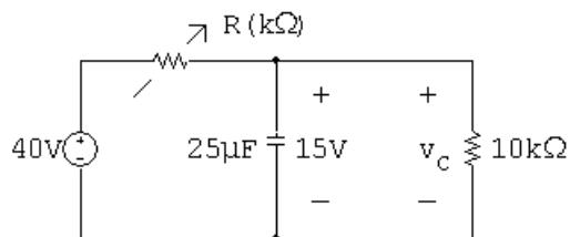
$$v_{Th} = \frac{10}{R+10}(40) = \frac{400}{R+10}; \quad R_{Th} = \frac{10R}{R+10} \text{ k}\Omega$$
