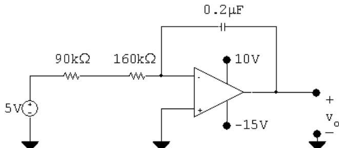
$$v_o = -\frac{1}{RC_f} \int_{32 \times 10^{-3}}^t 5 dy + 8 = -\frac{1}{RC_f} (5y) \Big|_{32 \times 10^{-3}}^t + 8 = -\frac{1}{RC_f} 5(t - 32 \times 10^{-3}) + 8$$
