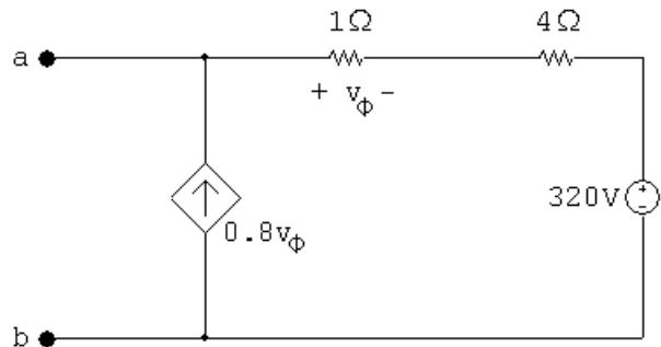
$$\frac{V_{Th} - 320}{5} - 0.8 \left( \frac{V_{Th} - 320}{5} \right) = 0 \quad V_{Th} = 320 \text{ V}$$
