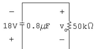
$$v_o = -18e^{-25t} \text{ V}, \quad t \geq 0$$
