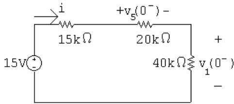
Find the current in the loop and use it to find the initial voltage drops across the two  $RC$  circuits:
