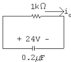
$$i_o(t) = \frac{24}{1 \times 10^3} e^{-t/\tau} = 24e^{-5000t} \text{ mA}, \quad t \geq 0^+$$
