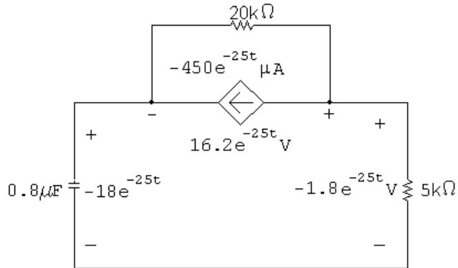
$$p_{ds} = (16.2e^{-25t})(-450 \times 10^{-6} e^{-25t}) = -7290 \times 10^{-6} e^{-50t} \text{ W}$$
