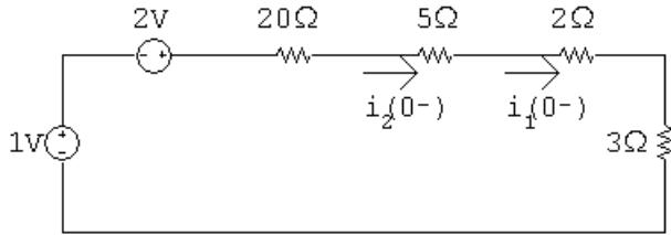
$$i_1(0^-) = i_2(0^-) = \frac{3 \text{ V}}{30 \Omega} = 100 \text{ mA}$$
