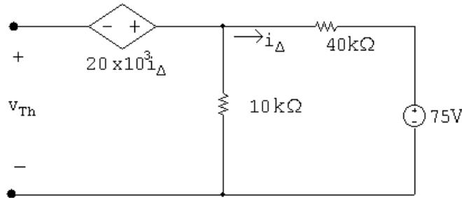
$$V_{Th} = -20 \times 10^3 i_\Delta + \frac{10}{50}(75) = -20 \times 10^3 \left( \frac{-75}{50 \times 10^3} \right) + 15 = 45 \text{ V}$$
