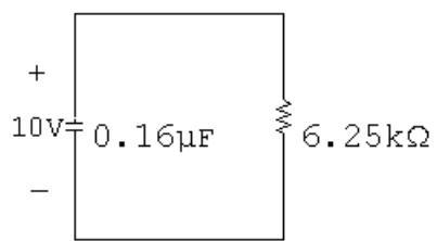
$$\tau = (6.25 \text{ k})(0.16 \mu) = 1 \text{ ms}; \quad 1/\tau = 1000; \quad v_o = 10e^{-1000(t - 0.05)} \text{ V}$$
