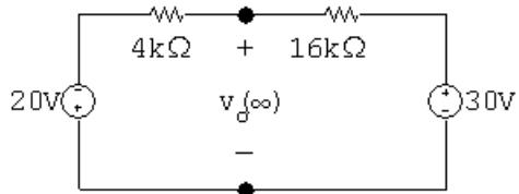
$$i = \frac{-50 \text{ V}}{20 \text{ k}\Omega} = -2.5 \text{ mA}$$
