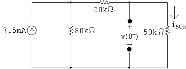
Find the voltage drop across the open circuit by finding the voltage drop across the  $50\text{k}\Omega$  resistor. First use current division to find the current through the  $50\text{k}\Omega$  resistor:
