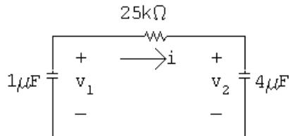
$$v_1 = \frac{-1}{10^{-6}} \int_0^t 1.6 \times 10^{-3} e^{-50x} dx + 40 = 32e^{-50t} + 8 \text{ V}, \quad t \geq 0$$
