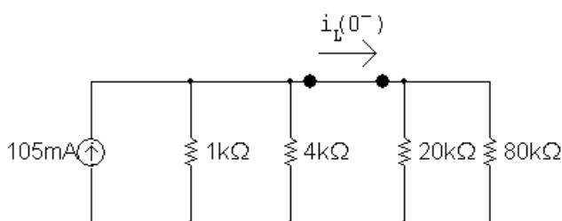
$$1\text{k}\Omega \parallel 4\text{k}\Omega = 0.8\text{k}\Omega$$
