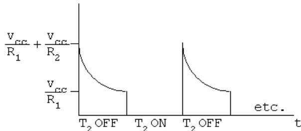
P 7.98 [a]  $t_{OFF2} = R_2 C_2 \ln 2 = 14.43 \times 10^3 (1 \times 10^{-9}) \ln 2 \cong 10 \mu s$
