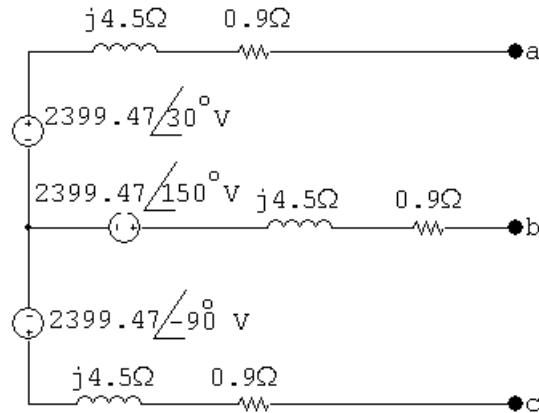
$$[\text{b}] \quad \mathbf{V}_{\text{ab}} = 2399.47/30^\circ - 2399.47/150^\circ = 2399.47\sqrt{3}/0^\circ = 4156/0^\circ \text{ V}$$
