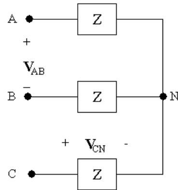
We know  $\mathbf{V}_{CN}$  and wish to find  $\mathbf{V}_{AB}$ . To do this, write a KVL equation to find  $\mathbf{V}_{BC}$ , and use the known phase angle relationship between  $\mathbf{V}_{AB}$  and  $\mathbf{V}_{BC}$  to find  $\mathbf{V}_{AB}$ .
