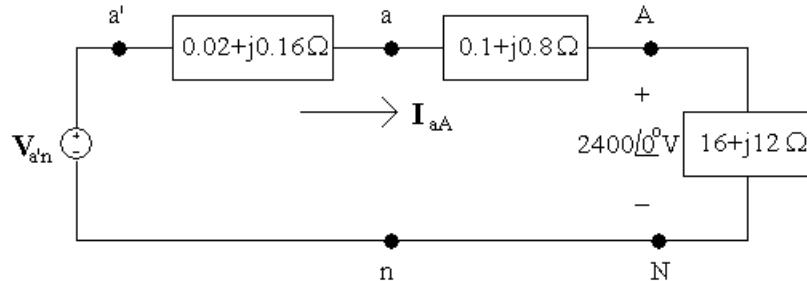
**[a]** We can find the line current using Ohm's law, since the a-phase line current is the current in the a-phase load. Then we can use the fact that  $\mathbf{I}_{aA}$ ,  $\mathbf{I}_{bB}$ , and  $\mathbf{I}_{cC}$  form a balanced set to find the remaining line currents. Note that since we were not given any phase angles in the problem statement, we can assume that the phase voltage given,  $\mathbf{V}_{AN}$ , has a phase angle of  $0^\circ$ .
