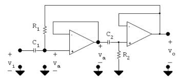
At low frequencies the capacitors appear as open circuits and hence the output voltage is zero. As the frequency increases the capacitor branches approach short circuits and  $v_a = v_i = v_o$ . Thus the circuit is a unity-gain, high-pass filter.
