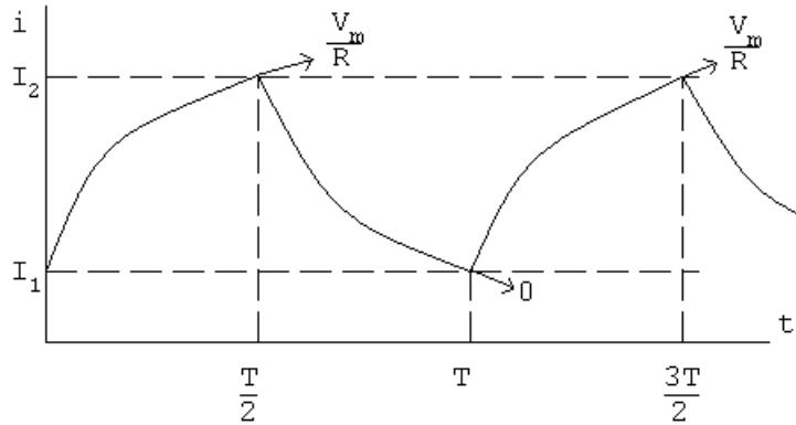
The steady-state current will alternate between  $I_1$  and  $I_2$  in exponential traces as shown. Assuming  $t = 0$  at the instant  $i$  increases toward  $(V_m/R)$ , we have
