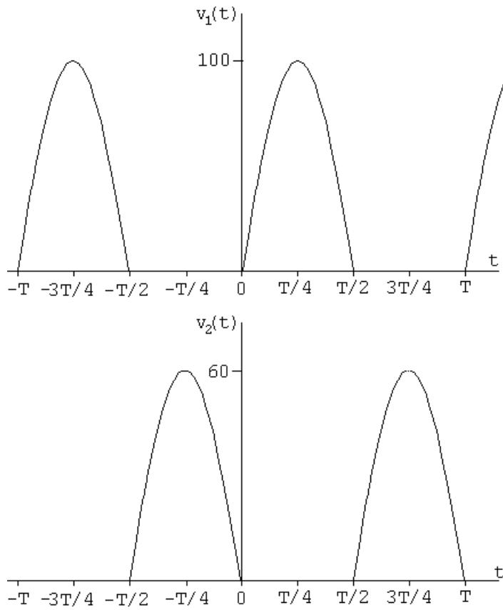
$$v_1(t) = \frac{100}{\pi} + 50 \sin \omega_o t - \frac{200}{\pi} \sum_{n=2,4,6}^{\infty} \frac{\cos n\omega_o t}{(n^2 - 1)} V$$
